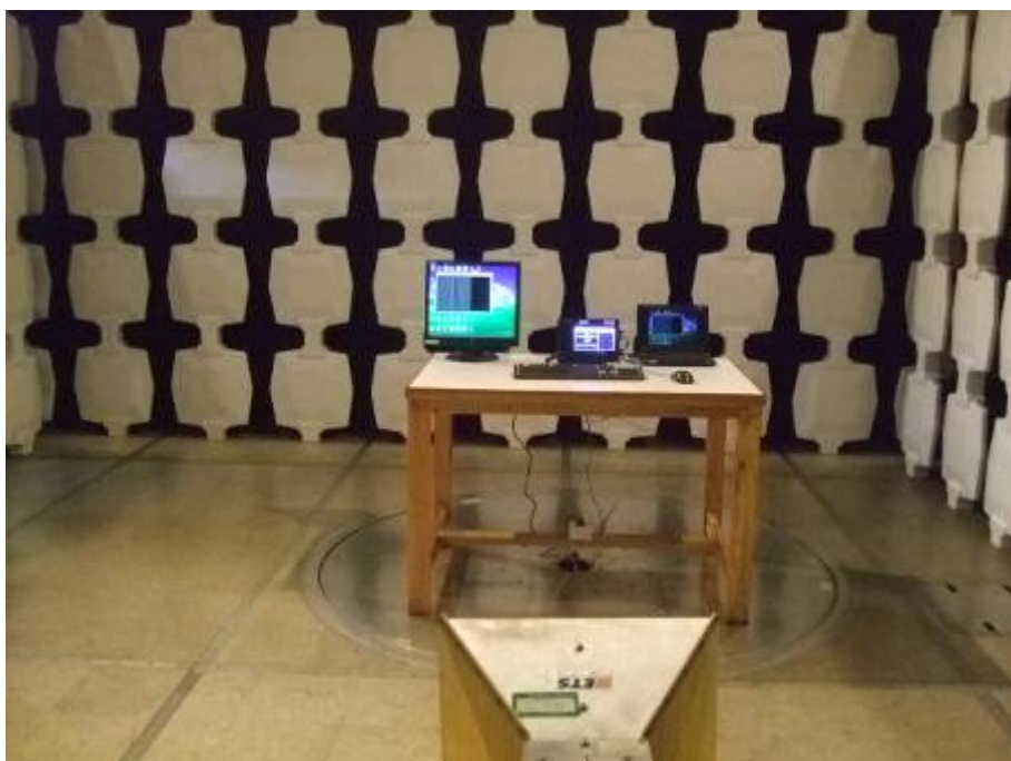
Radiated Emission Test Set-up (Above 1GHz)
