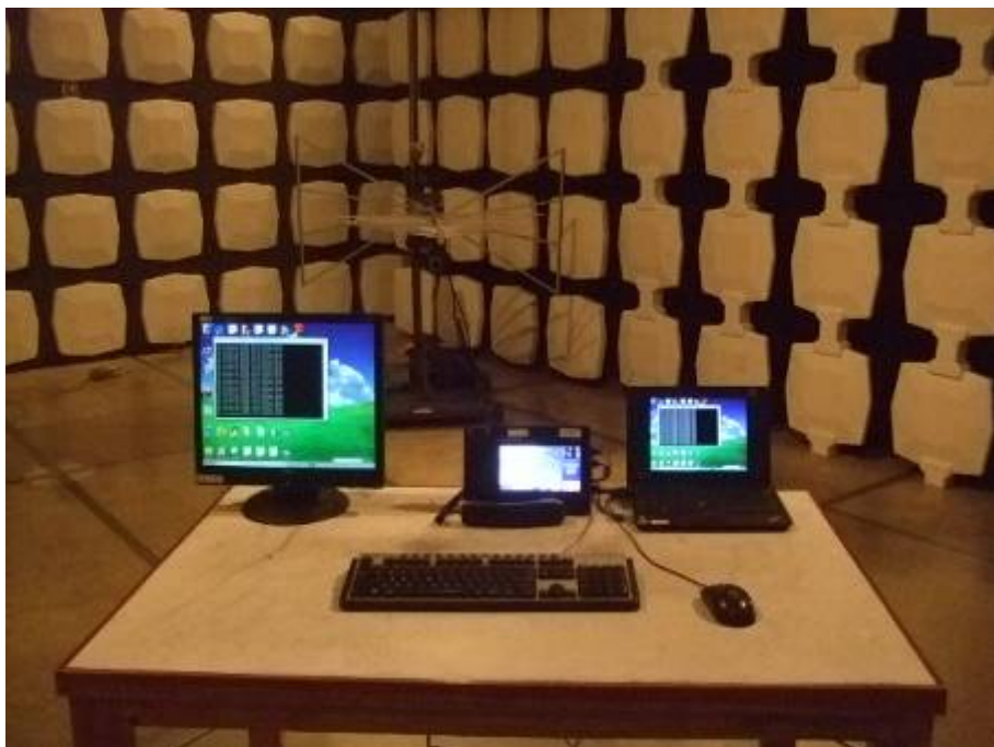
Radiated Emission Test Set-up (Below 1GHz)
