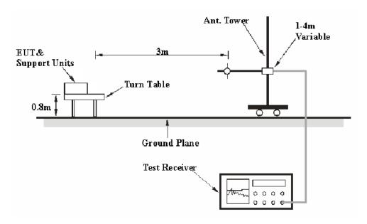
The radiated emission tests were performed in the 3 meters chamber B test site, using the setup accordance with the ANSI C63.4-2009. The specification used was the FCC Part 15 Class B limits.
