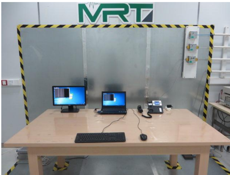
Conducted Emission Test Set-up- Front View
