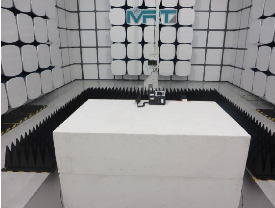
Radiated Emission Test Set-up (1-18GHz)
