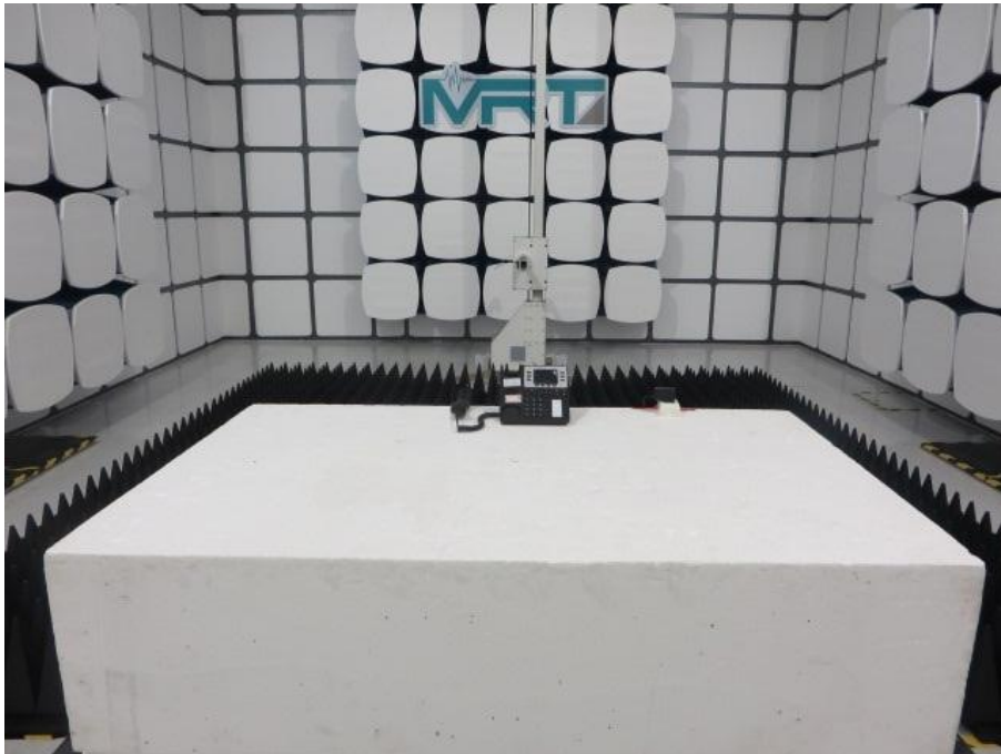
Radiated Emission Test Set-up (18-40GHz)
