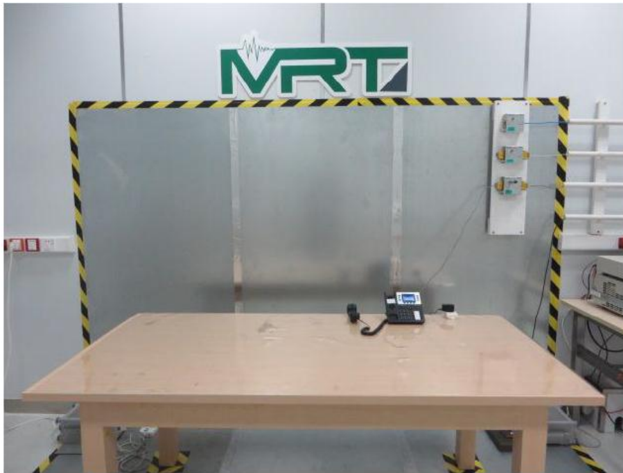
Conducted Emission Test Set-up- Front View
