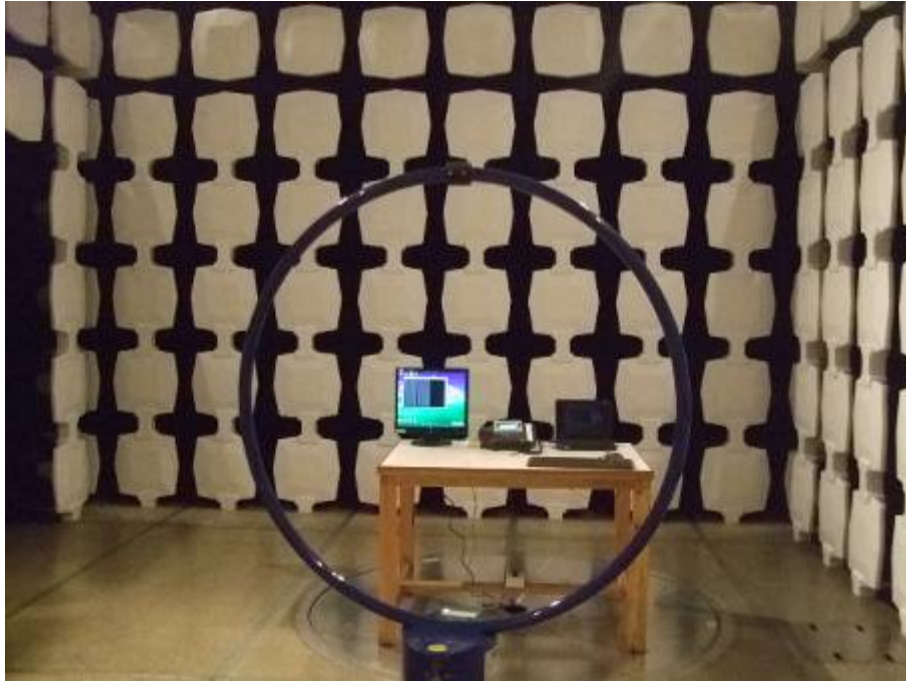
Radiated Emission Test Set-up(9KHz-30MHz)
