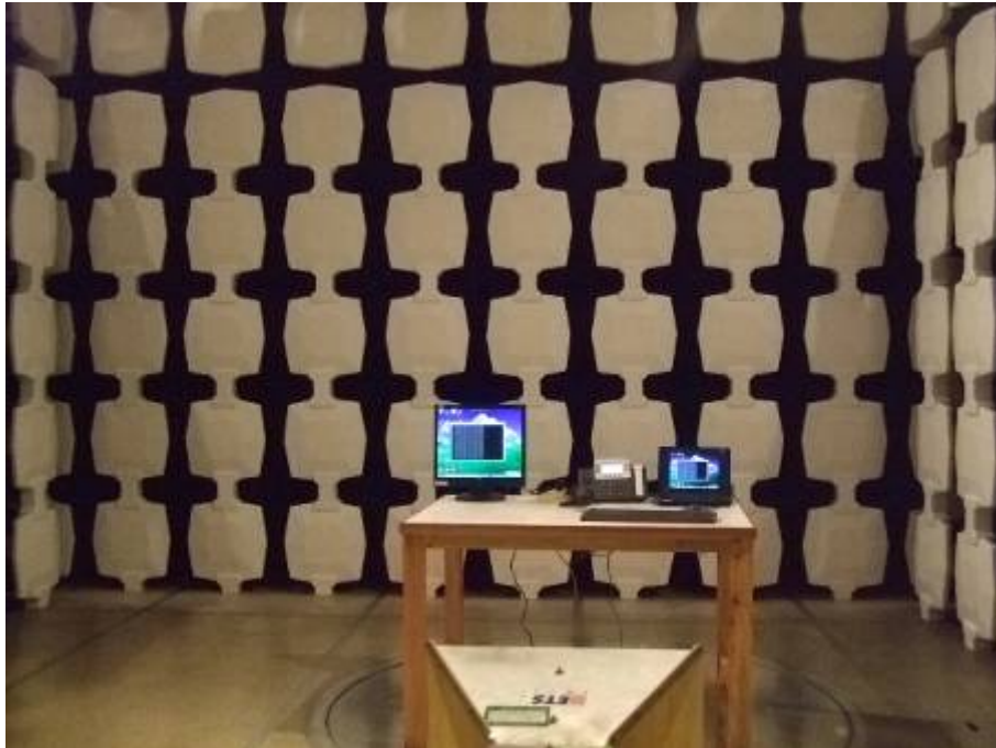
Radiated Emission Test Set-up(Above 1GHz)
