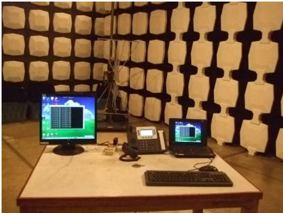
Radiated Emission Test Set-up(Below 1GHz)
