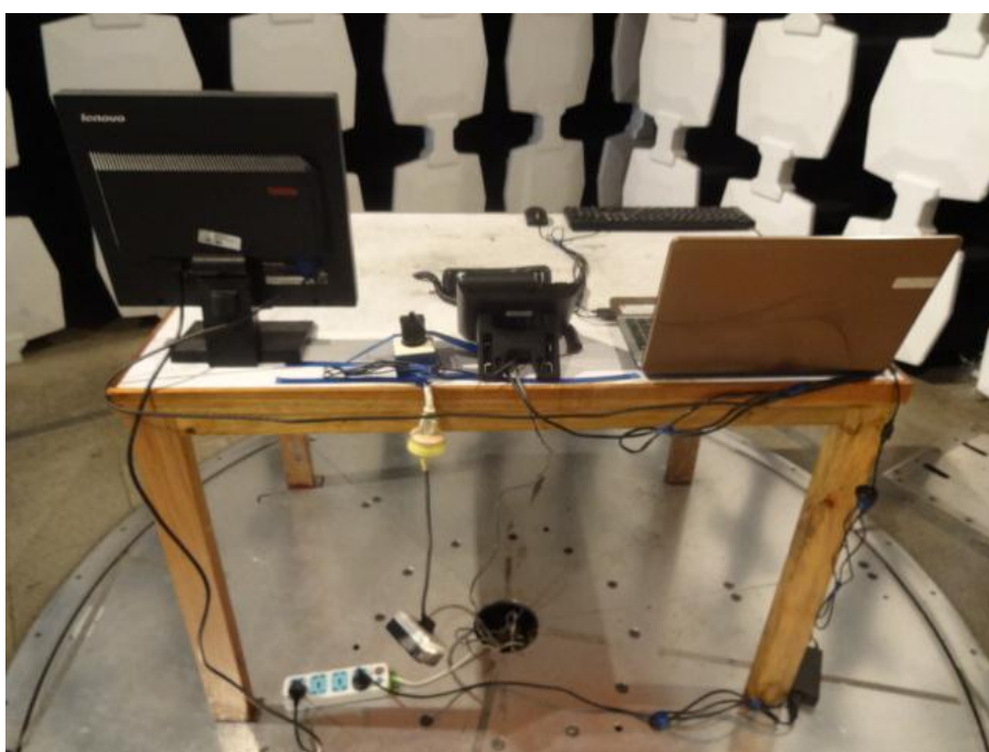
Radiated Emission Test Set-up (Rear View)
