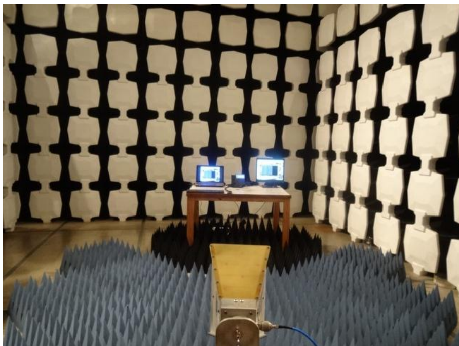
Radiated Emission Test Set-up(Above 1GHz)
