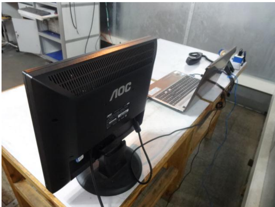
Conducted Emission Test Set-up -Rear view
