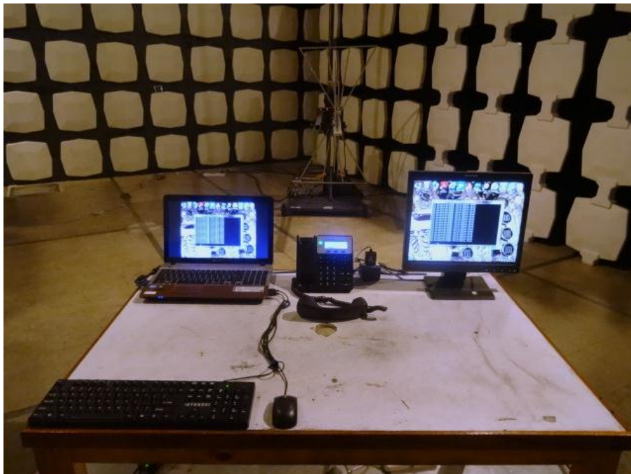
Radiated Emission Test Set-up(30-1000MHz)
