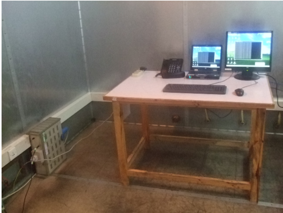
Conducted Emission Test Set-up
