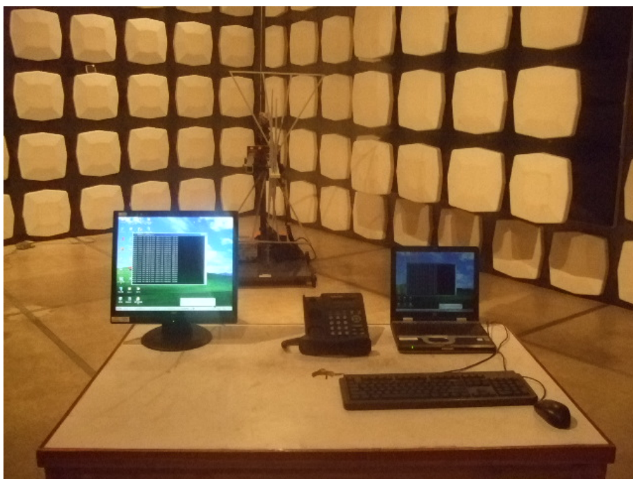
Radiated Emission Test Set-up(30-1000MHz)
