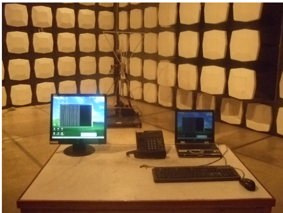
Radiated Emission Test Set-up(30-1000MHz)
