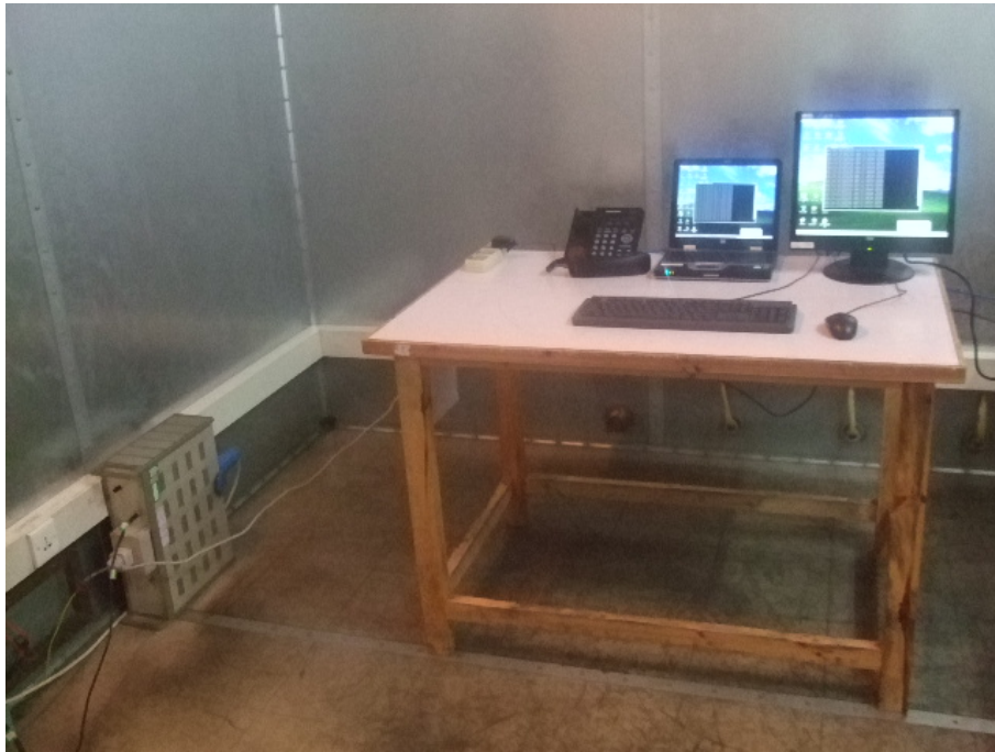
Conducted Emission Test Set-up
