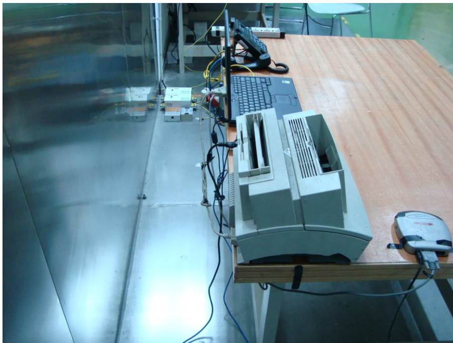
Conduction Emissions - Side View (Powered by AC/DC adapter)
