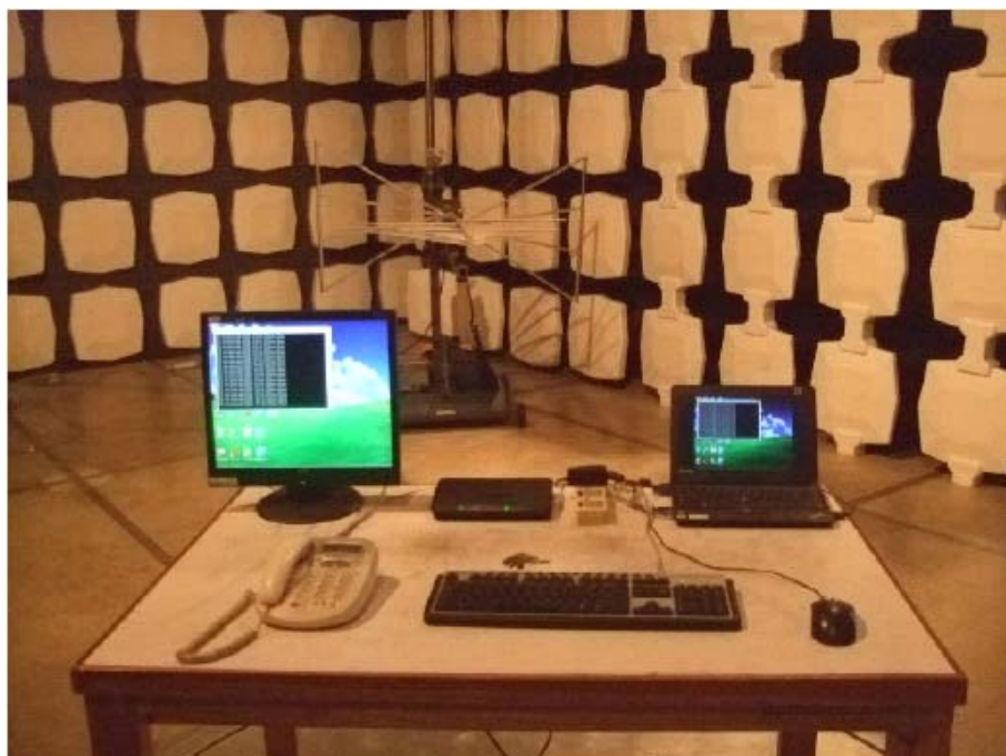
Radiated Emission Test Set-up (Below 1GHz)
