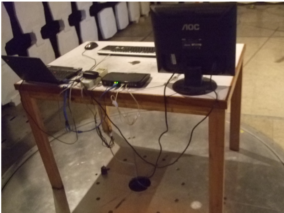
Radiated Emission Test Set-up (Rear view)
