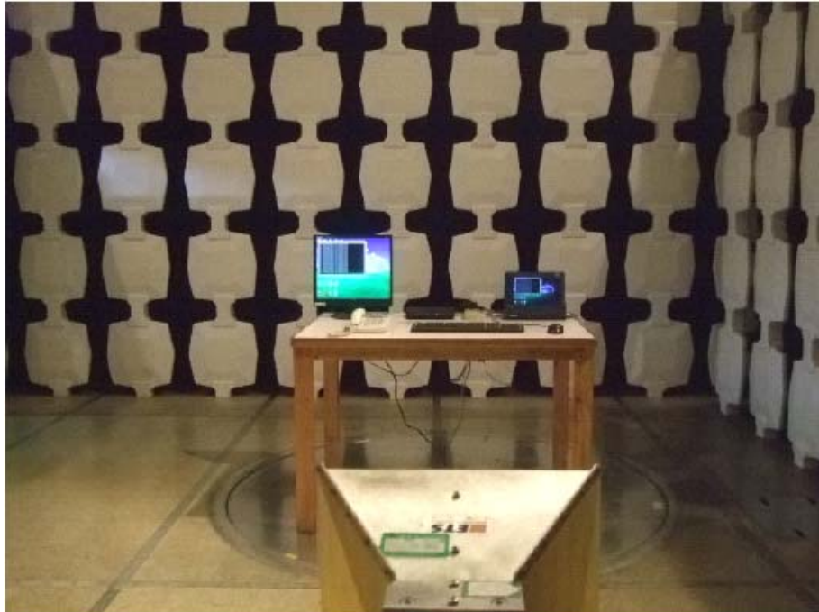
Radiated Emission Test Set-up (Above 1GHz)
