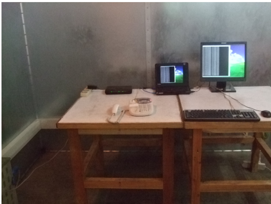
Conducted Emission Test Set-up -Front view
