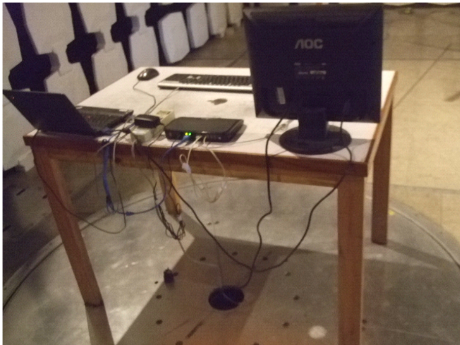
Radiated Emission Test Set-up (rear view)
