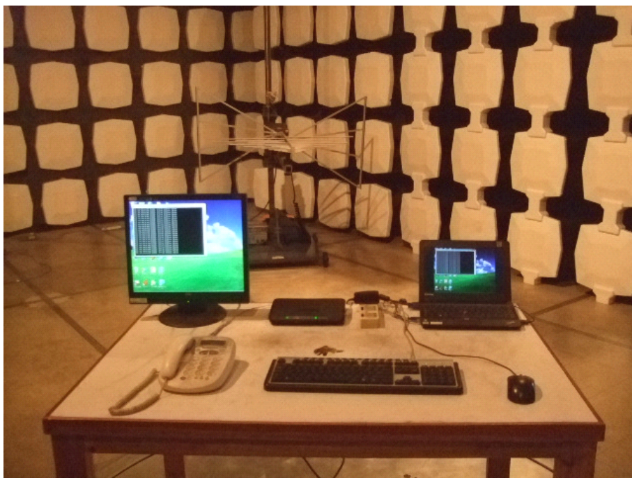
Radiated Emission Test Set-up (Below 1GHz)
