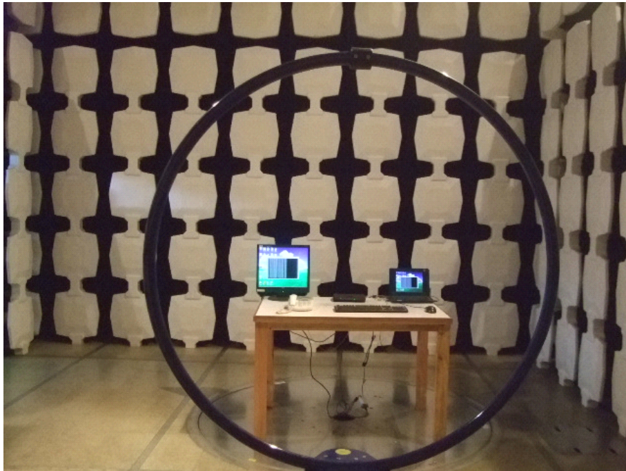
Radiated Emission Test Set-up (9KHz-30MHz)
