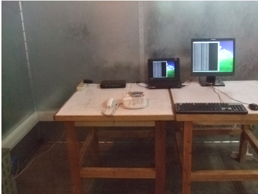
Conducted Emission Test Set-up -front view
