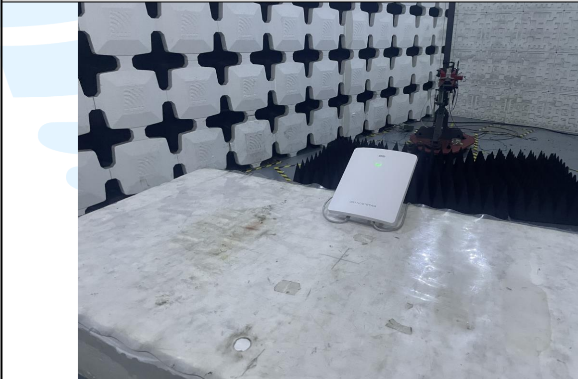
Radiated emission Test Setup-2 (Above 1 GHz)
