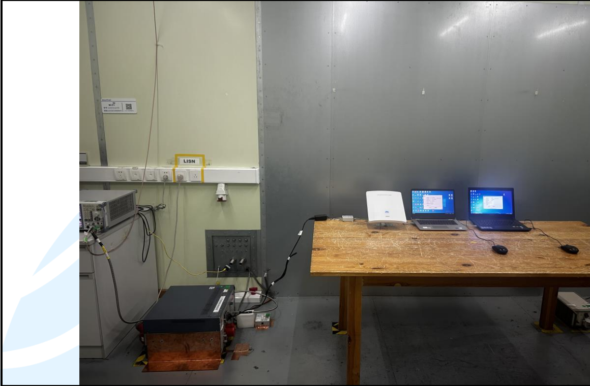
Conducted Emission Test Setup-3
