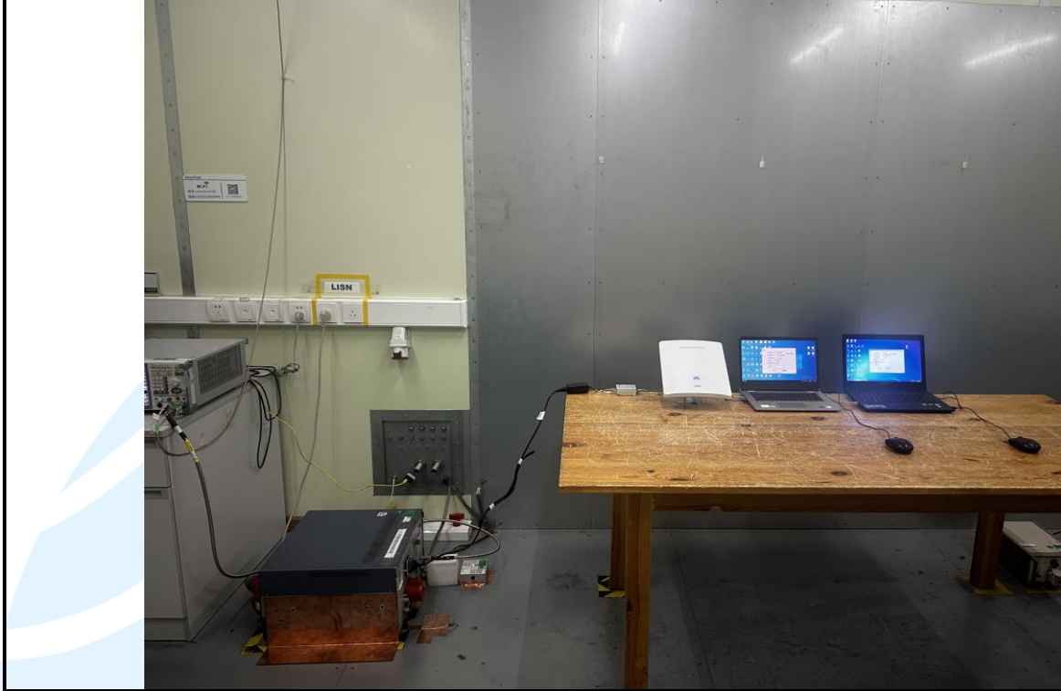
Conducted Emission Test Setup
