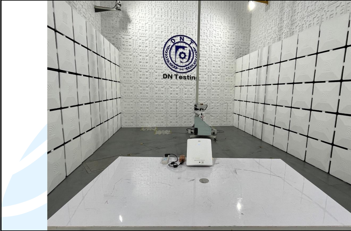
Radiated emission Test Setup (30 MHz~1 GHz)
