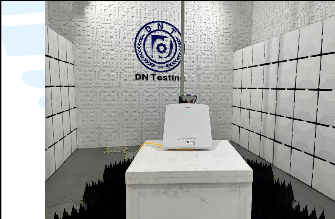
Radiated emission Test Setup (Above 1 GHz)
