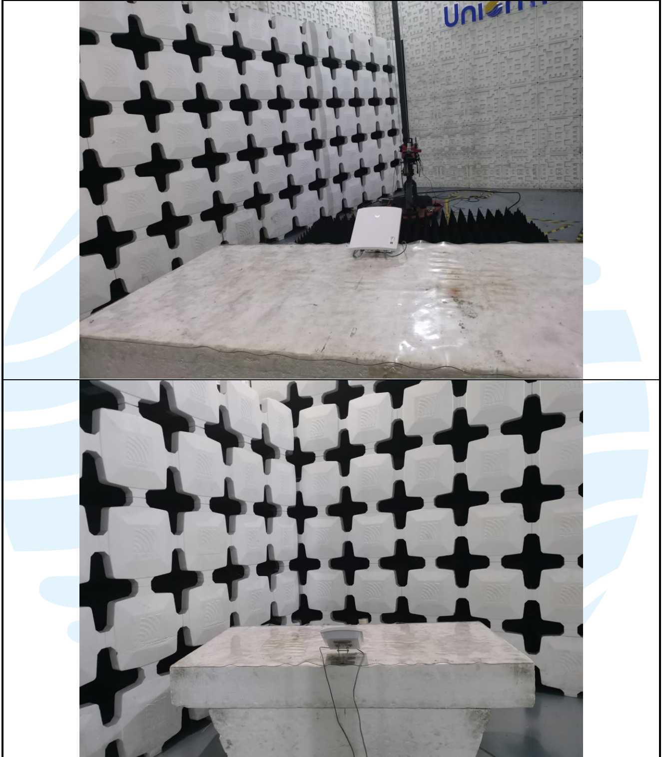
Radiated emission Test Setup-2 (Above 1 GHz)
