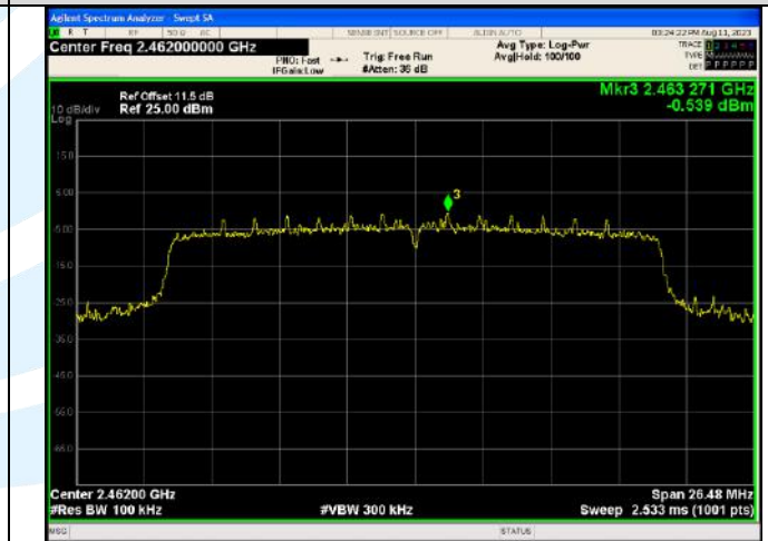
In-Band Reference Level IEEE 802.11ax_Channel 11_20MHz_Antenna 1_RU&Index SU
