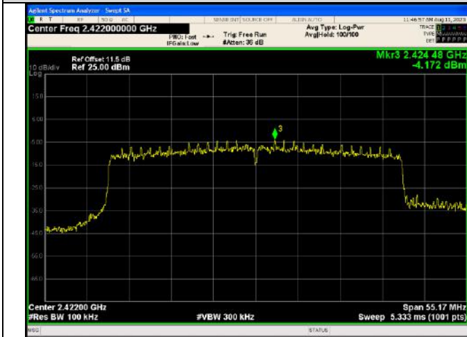
In-Band Reference Level IEEE 802.11ax_Channel 3_40MHz_Antenna 0_RU&Index SU
