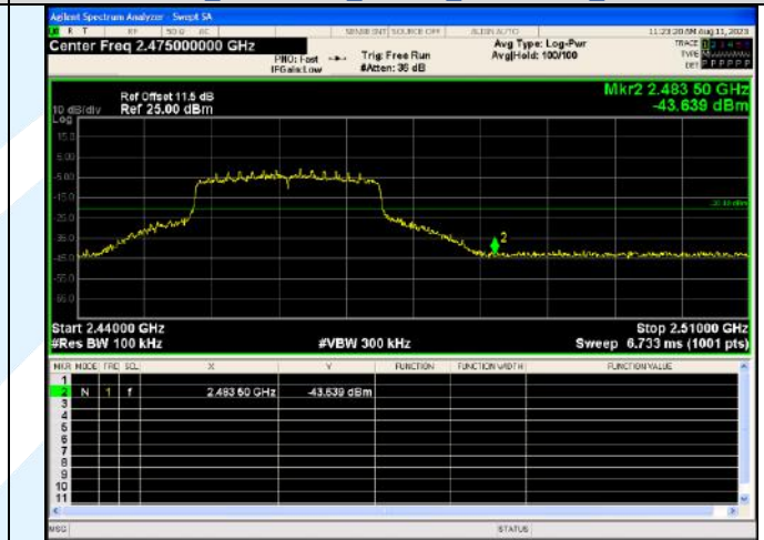
Out Of Band Emission IEEE 802.11ax_Channel 11_20MHz_Antenna 0_RU&Index SU
