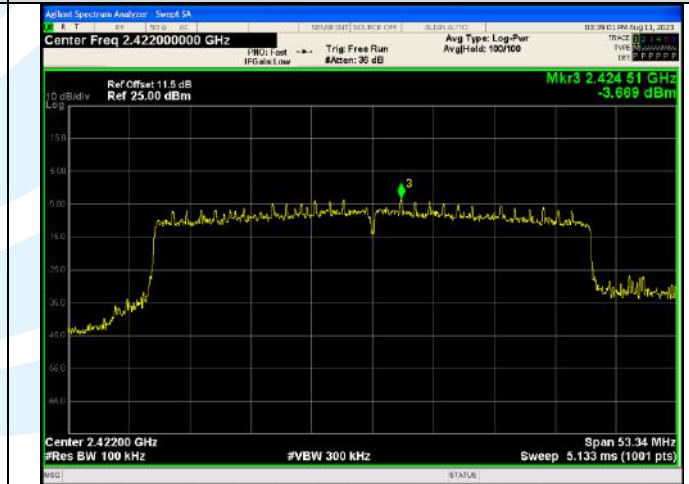
In-Band Reference Level IEEE 802.11ax_Channel 3_40MHz_Antenna 1_RU&Index SU
