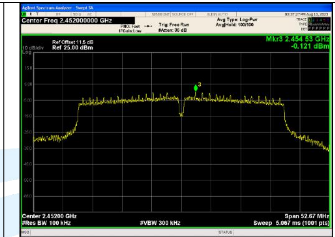
In-Band Reference Level IEEE 802.11n Channel 9 40MHz Antenna 1
