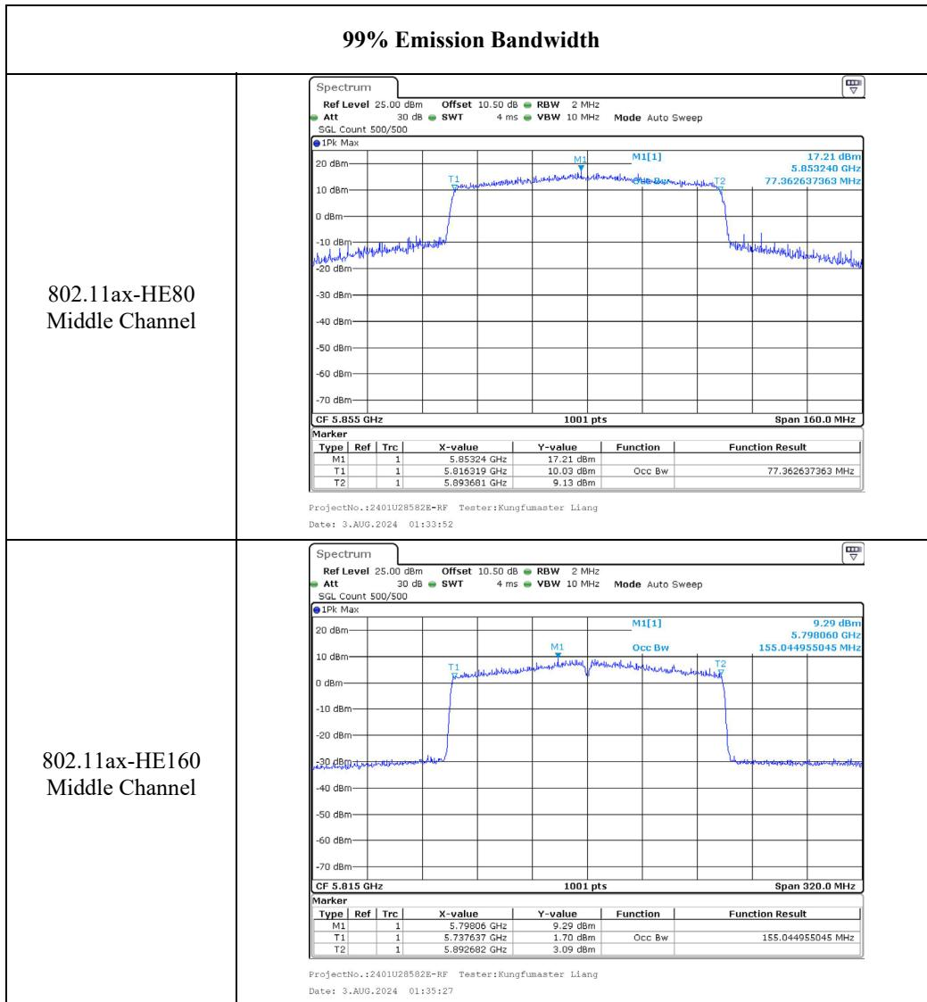
Note: The test data and plots of 5150-5250MHz, 5250-5350MHz, 5470-5725MHz and 5725-5850MHz band please refer to the Appendix.
