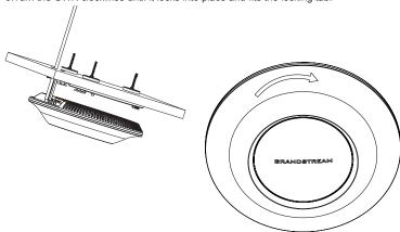
Note: Ceiling mounting is recommended for optimal coverage performance.
