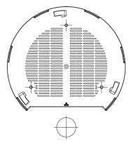
3. Insert screw anchors into the 5.5 mm holes. Attach the mounting bracket to the wall by inserting the screws into the anchors.
