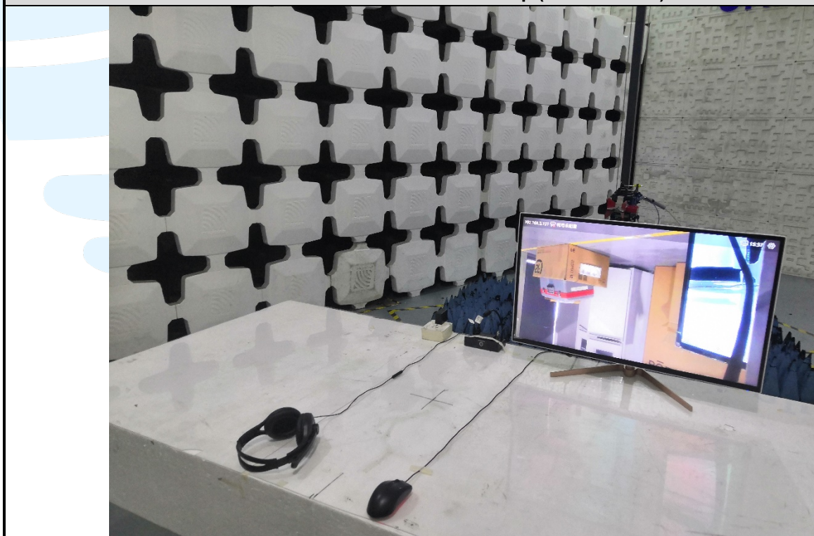
Radiated emission Test Setup (Above 1 GHz)
