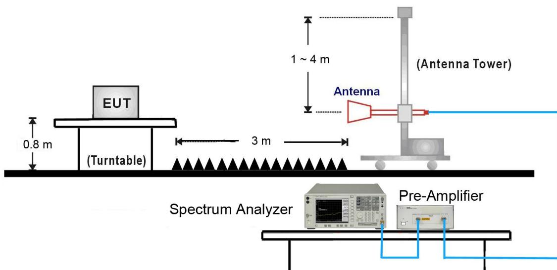
18GHz ~40GHz Test Setup:
