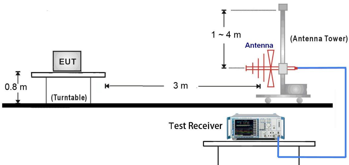
1GHz ~ 25GHz Test Setup:
