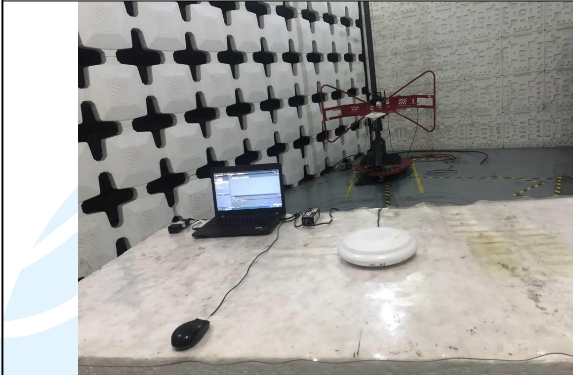
Radiated emission Test Setup (30 MHz~1 GHz)
