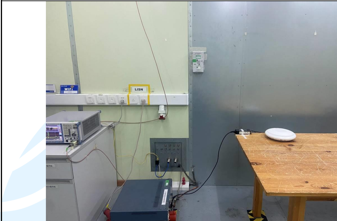
Conducted Emission Test Setup
