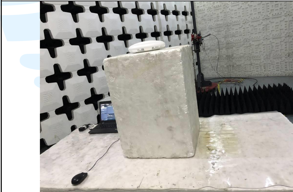
Radiated emission Test Setup (Above 1 GHz)
