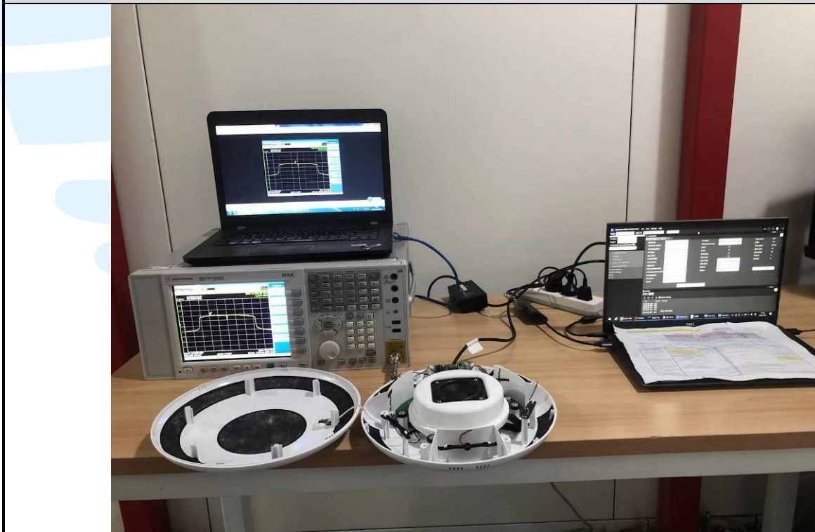
RF Conducted Test Setup
