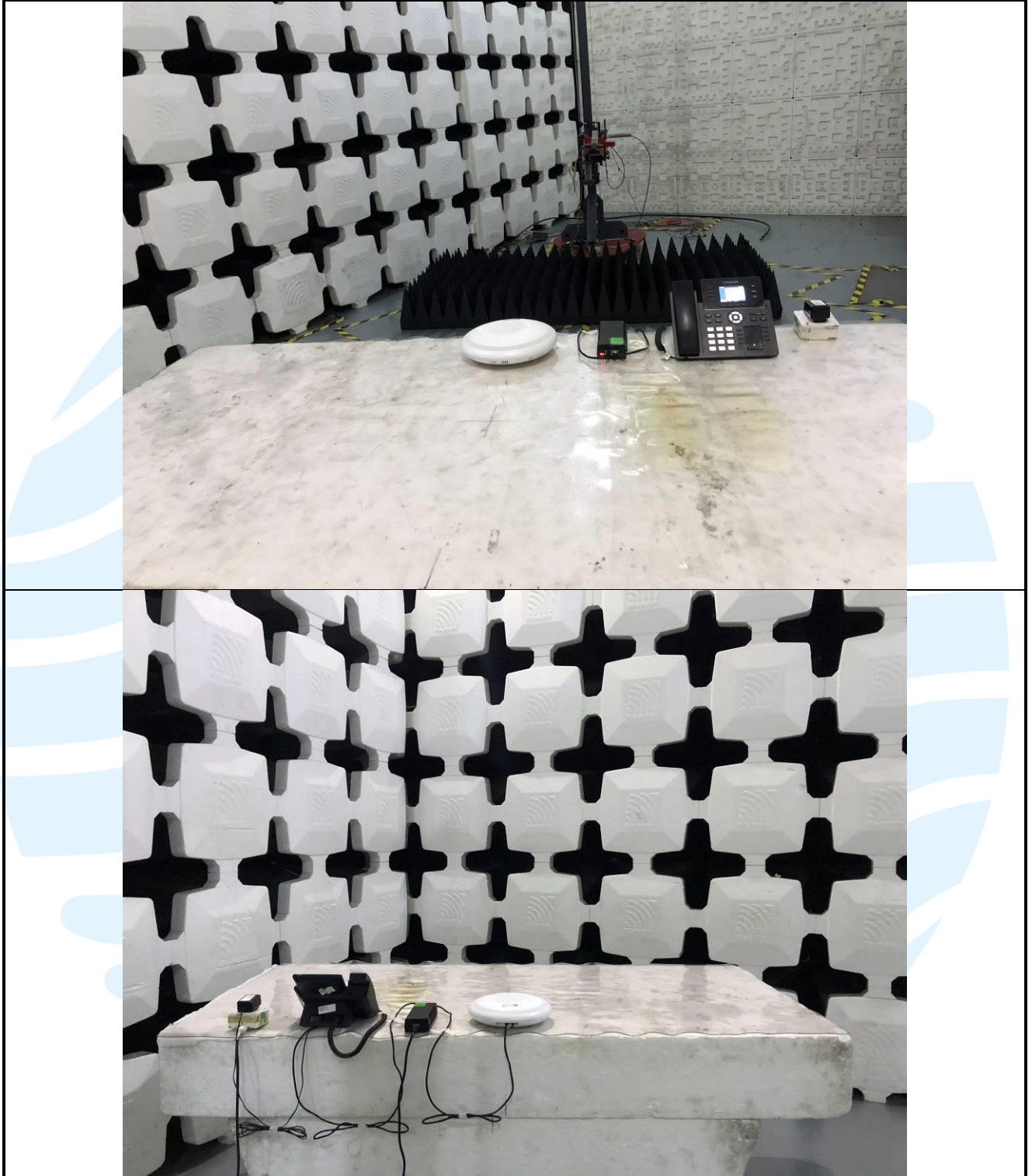
Radiated emission Test Setup-2 (Above 1 GHz)
