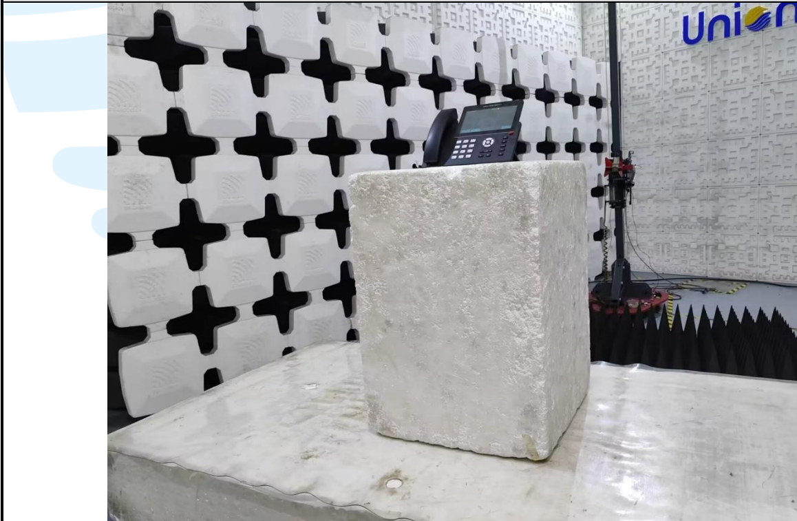
Radiated emission Test Setup (Above 1 GHz)
