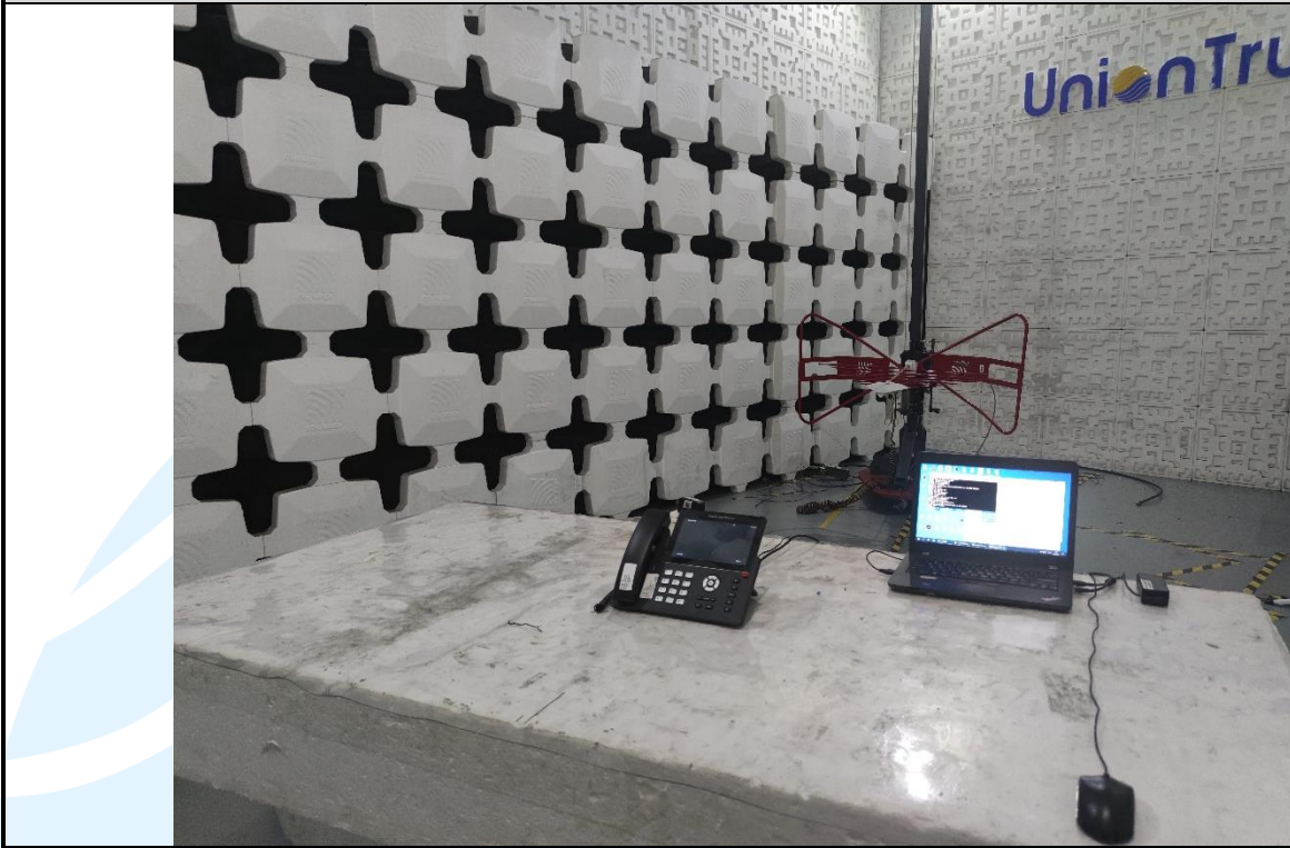
Radiated emission Test Setup (30 MHz~1 GHz)
