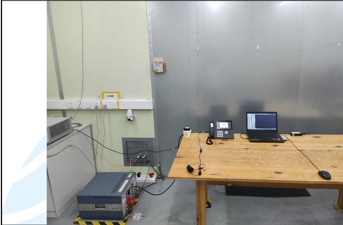
Conducted Emission Test Setup
