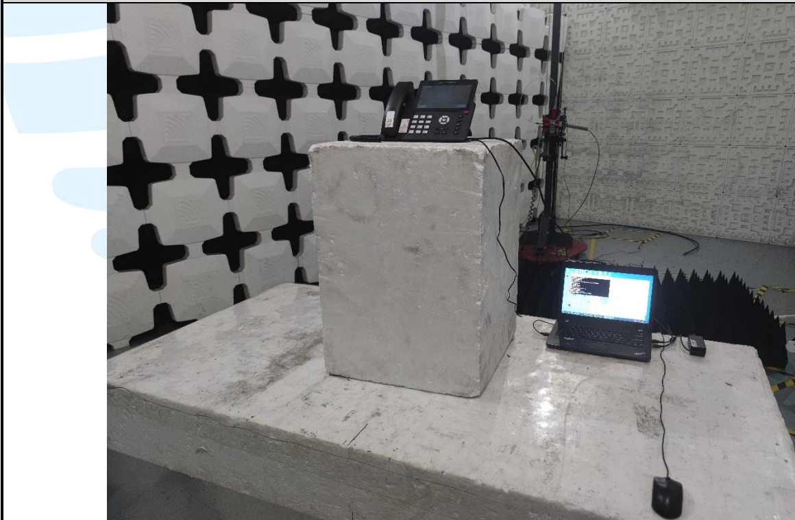
Radiated emission Test Setup (Above 1 GHz)
