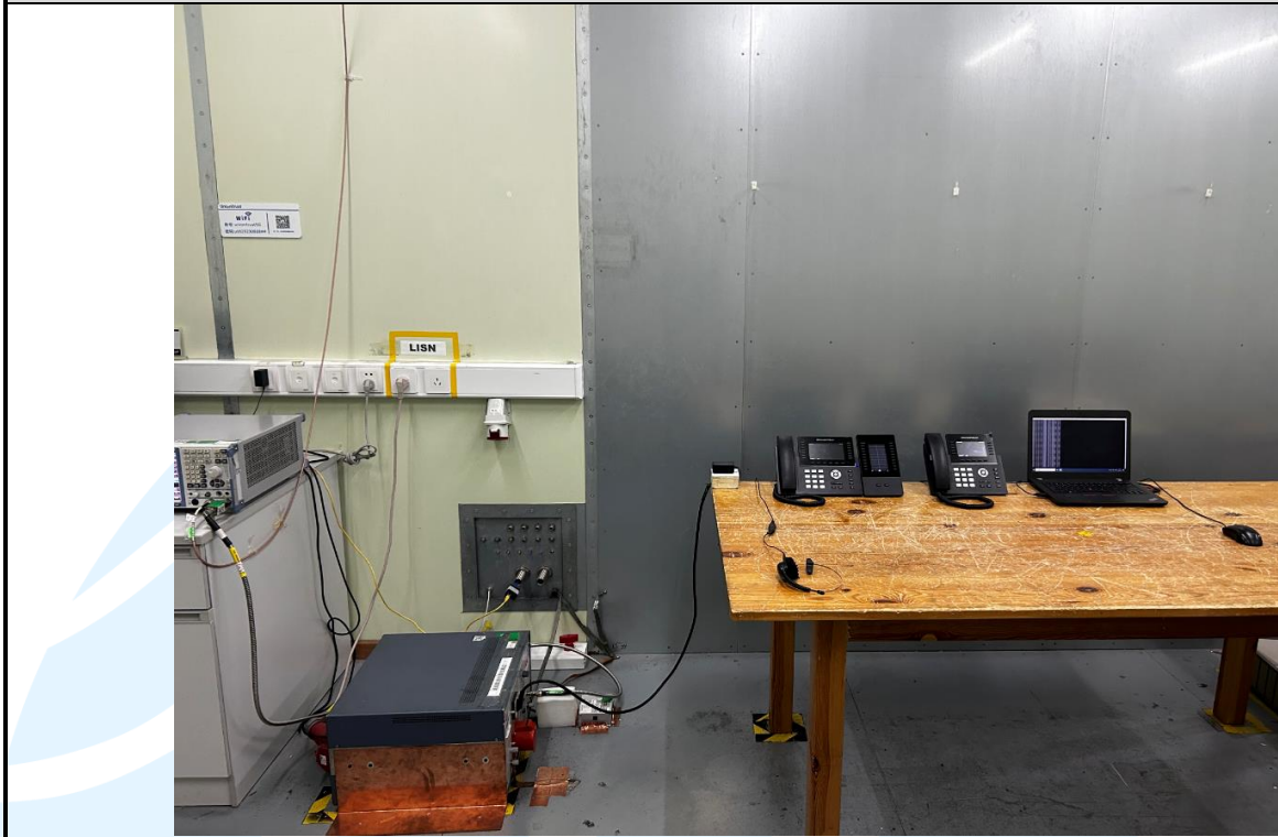
Conducted Emission Test Setup
