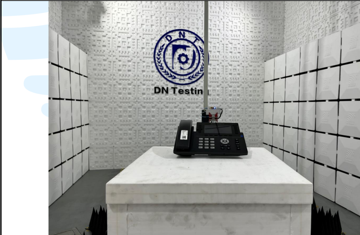
Radiated emission Test Setup (Above 1 GHz)
