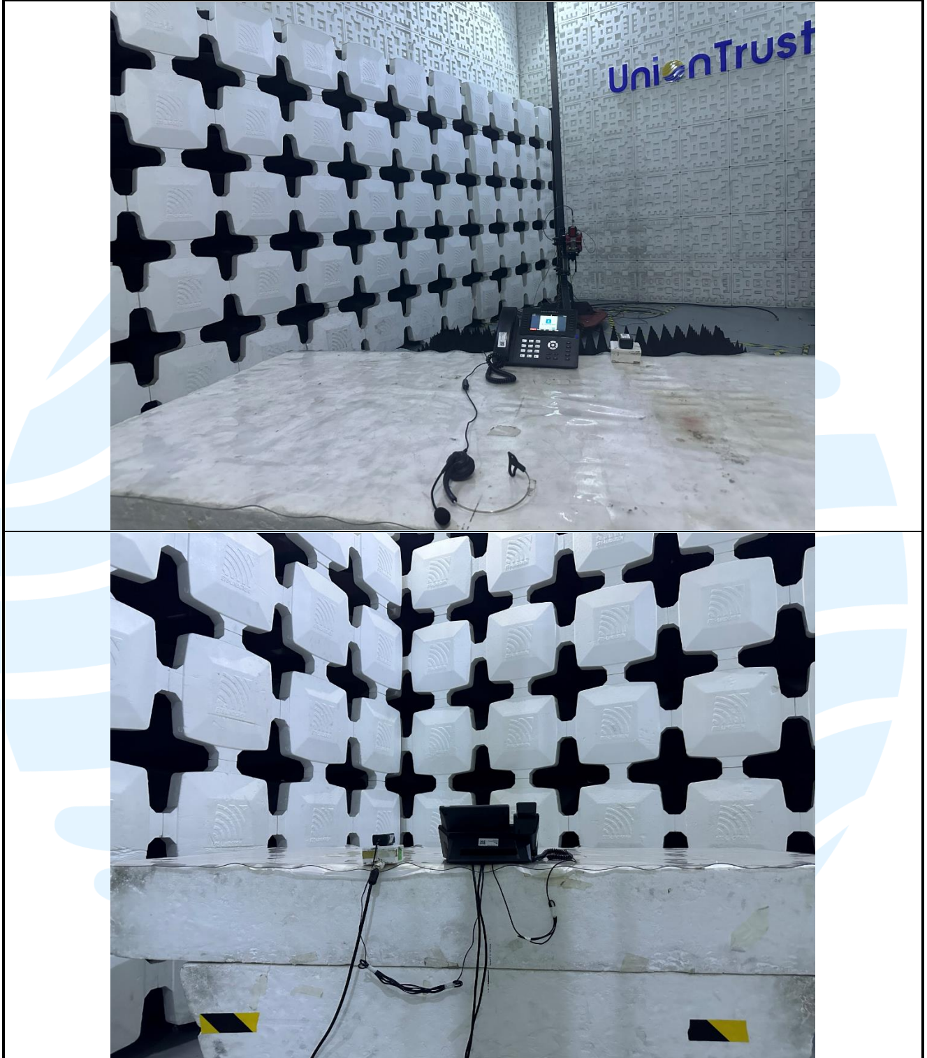
Radiated emission Test Setup-2 (Above 1 GHz)
