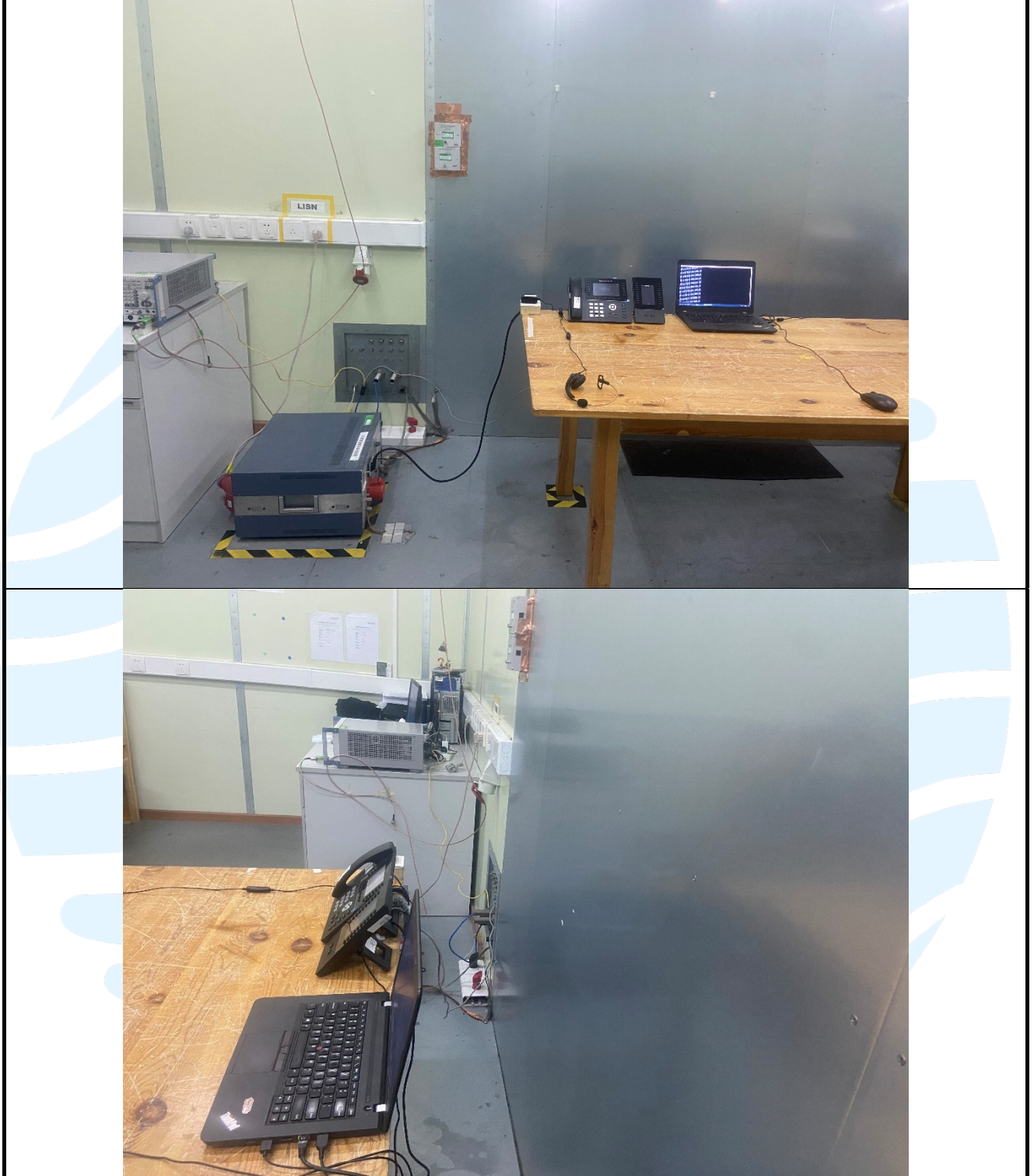
Conducted Emission (AC Port) Test Setup-5
