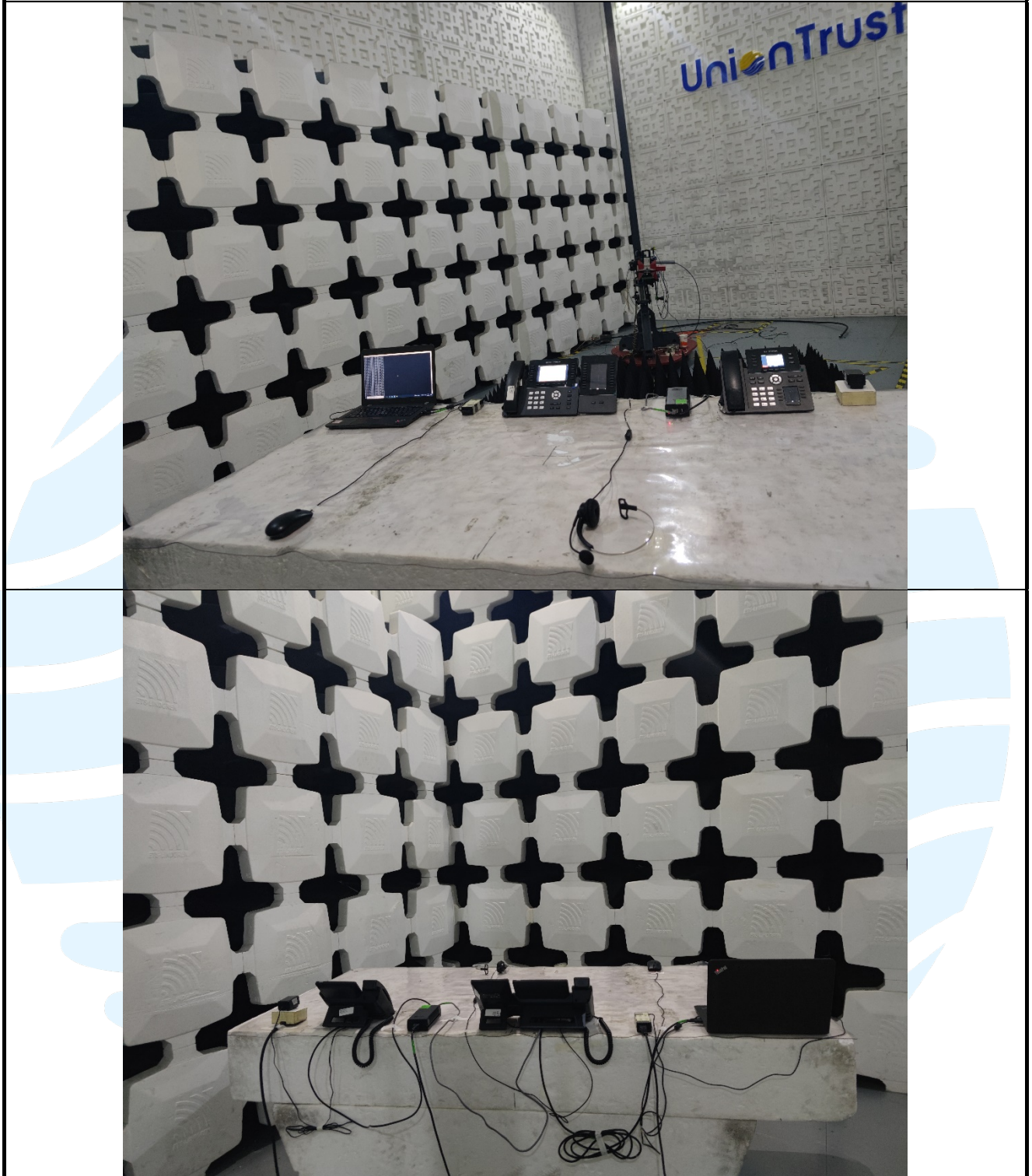
Radiated emission (PoE Port) Test Setup-2 (Above 1 GHz)
