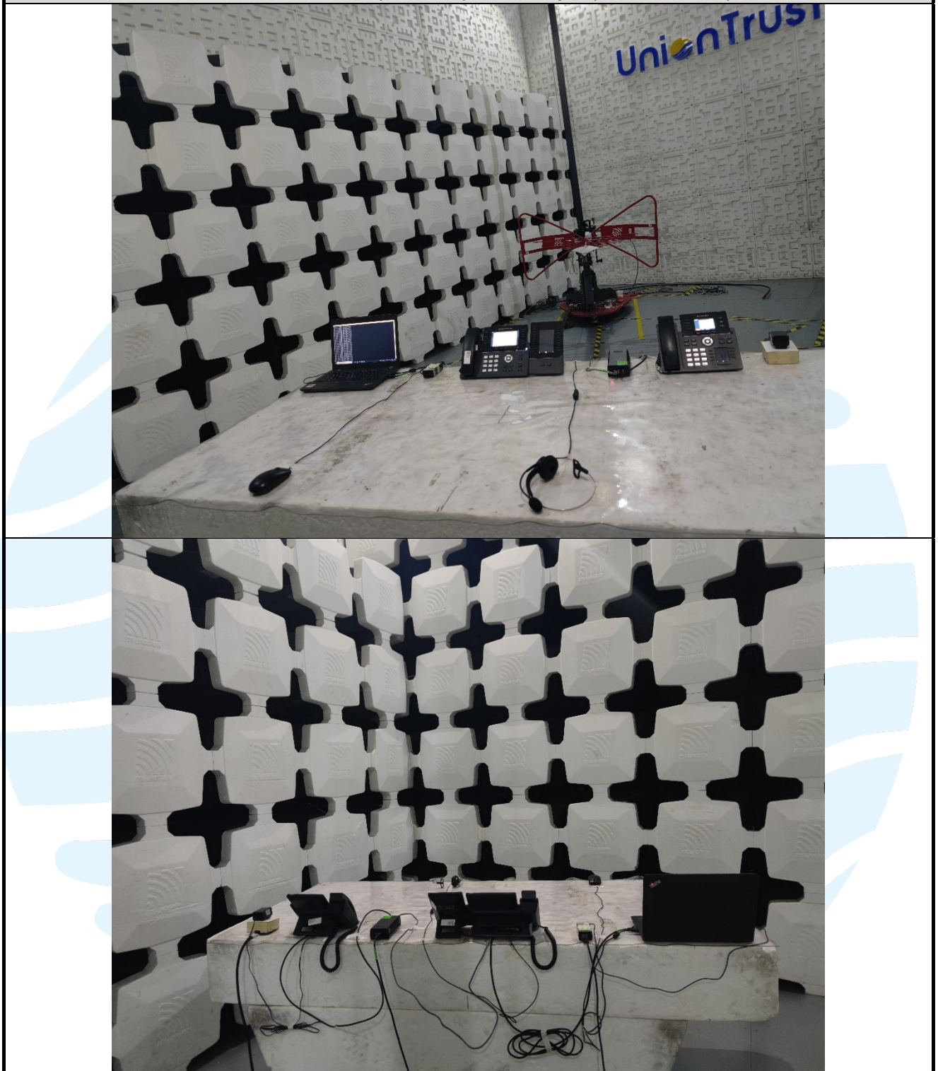
Radiated emission (PoE Port) Test Setup-3 (30 MHz~1 GHz)
