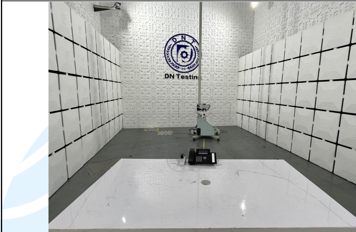
Radiated emission Test Setup (30 MHz~1 GHz)
