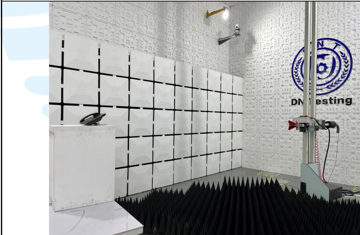
Radiated emission Test Setup (Above 1 GHz)
