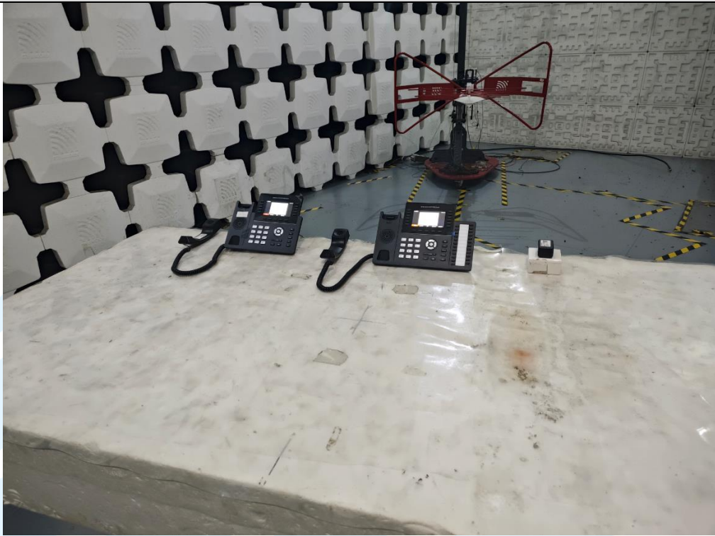
Radiated emission Test Setup-1 (30 MHz~1 GHz)
