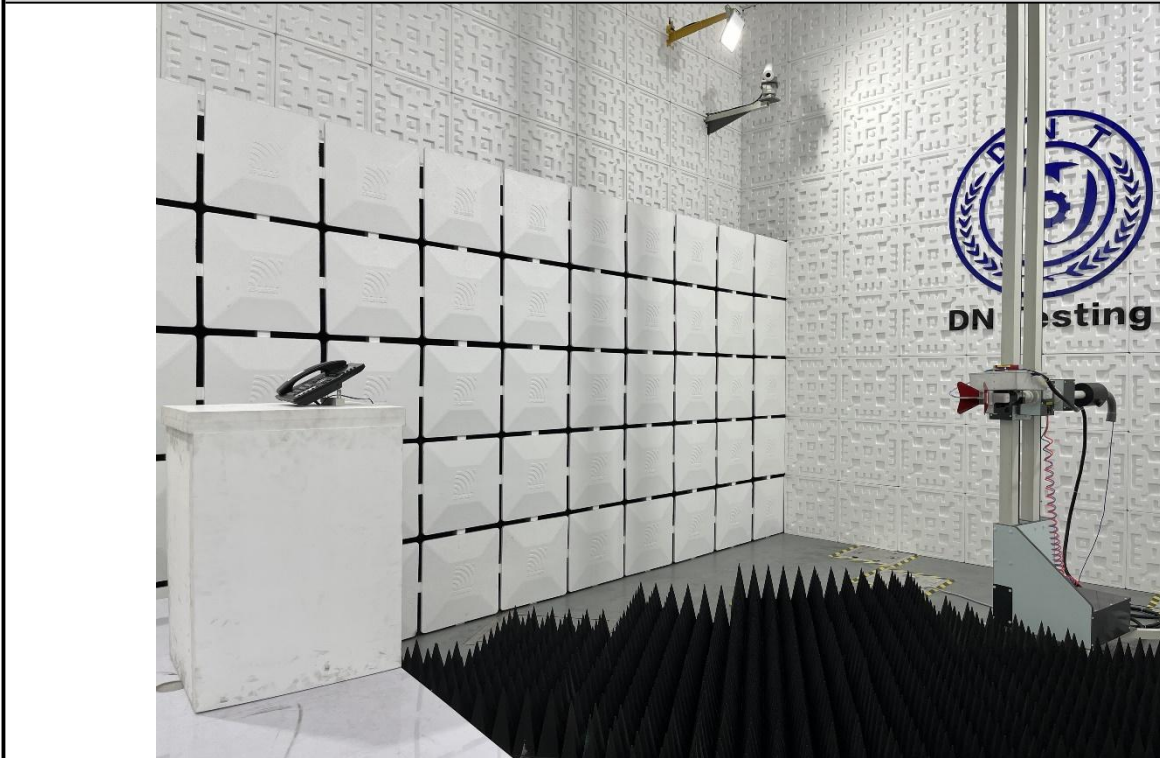
Radiated emission Test Setup (Above 1 GHz)
