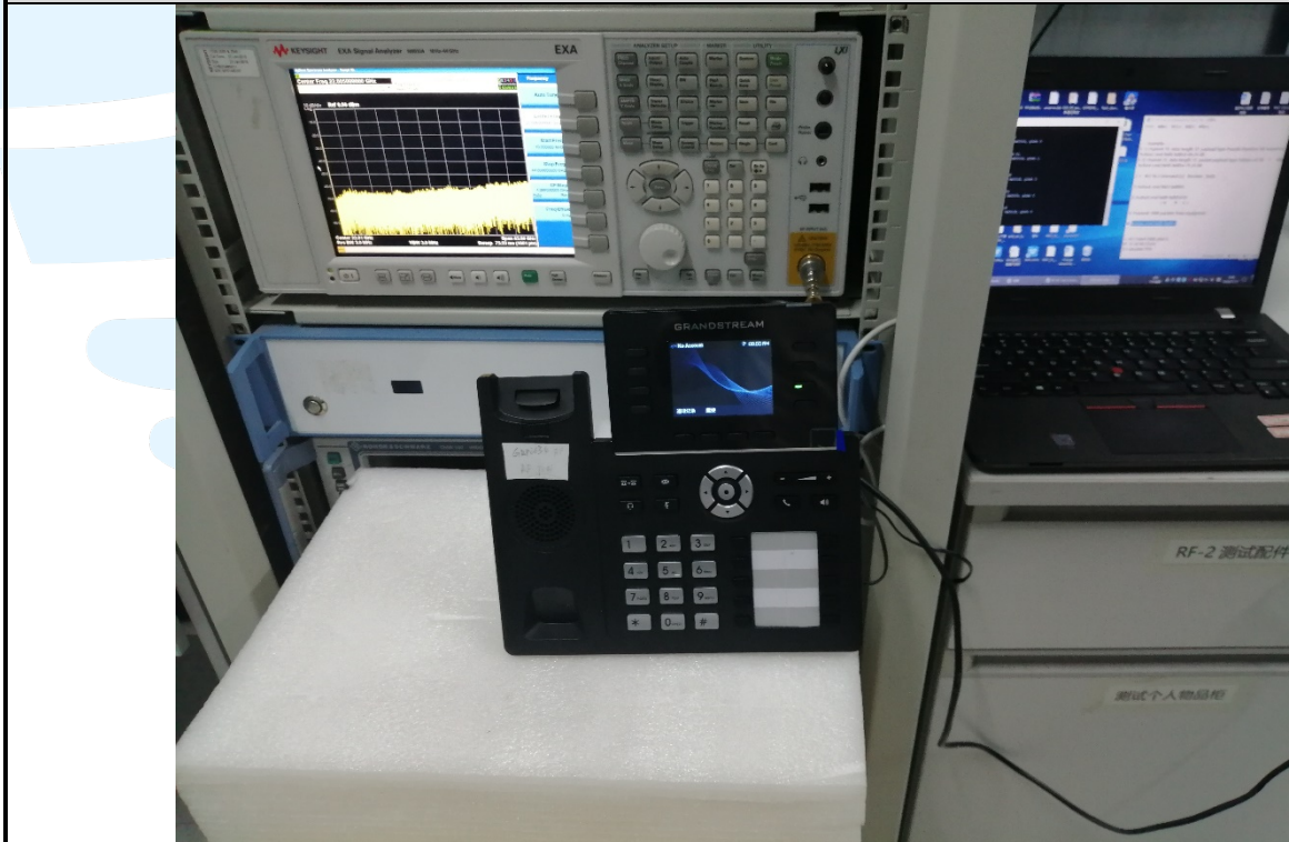
RF Conducted Test Setup
