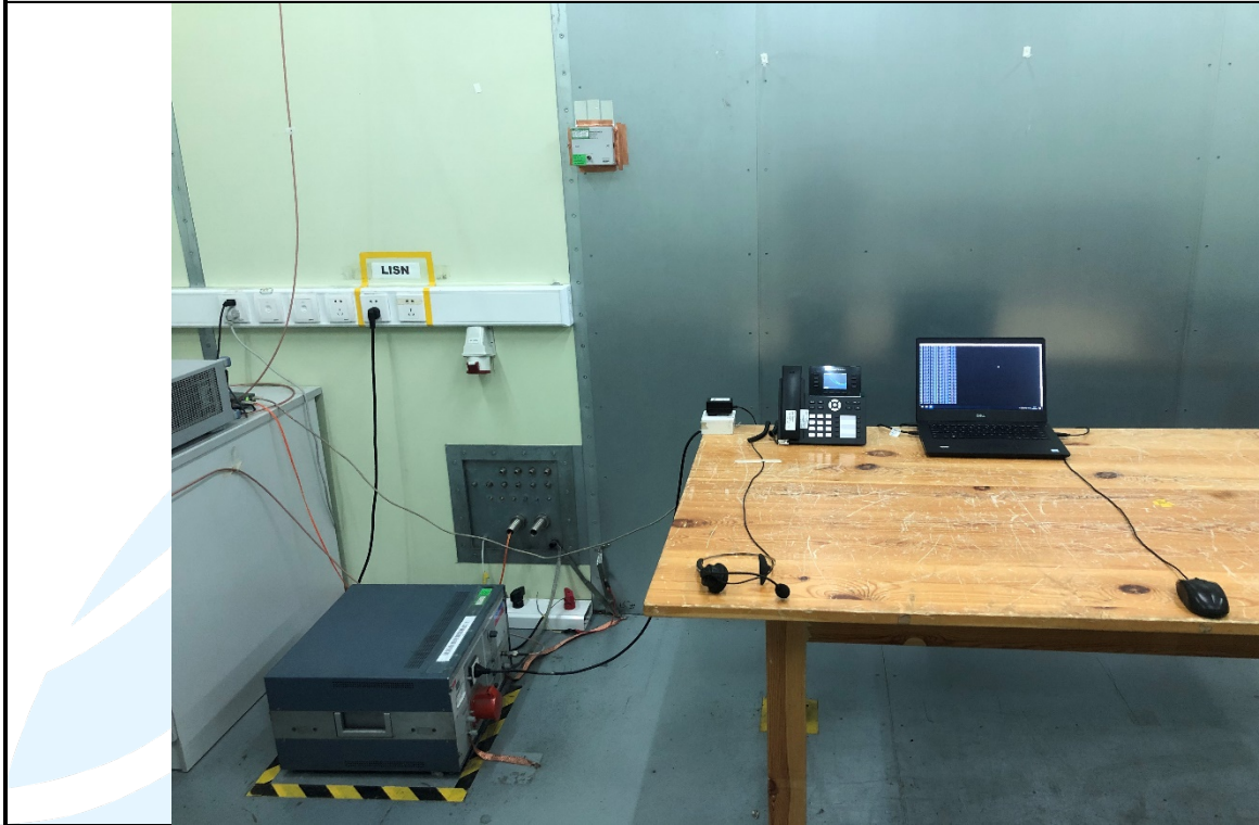
Conducted Emission Test Setup
