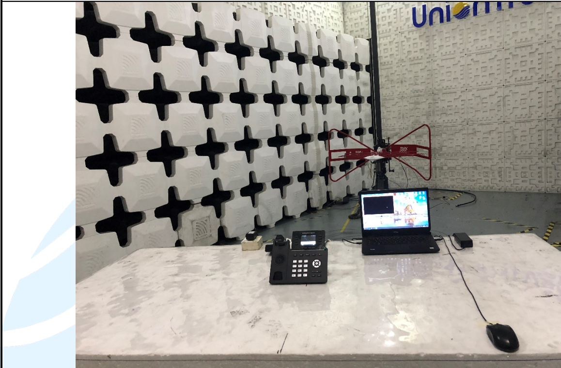
Radiated emission Test Setup (30 MHz~1 GHz)
