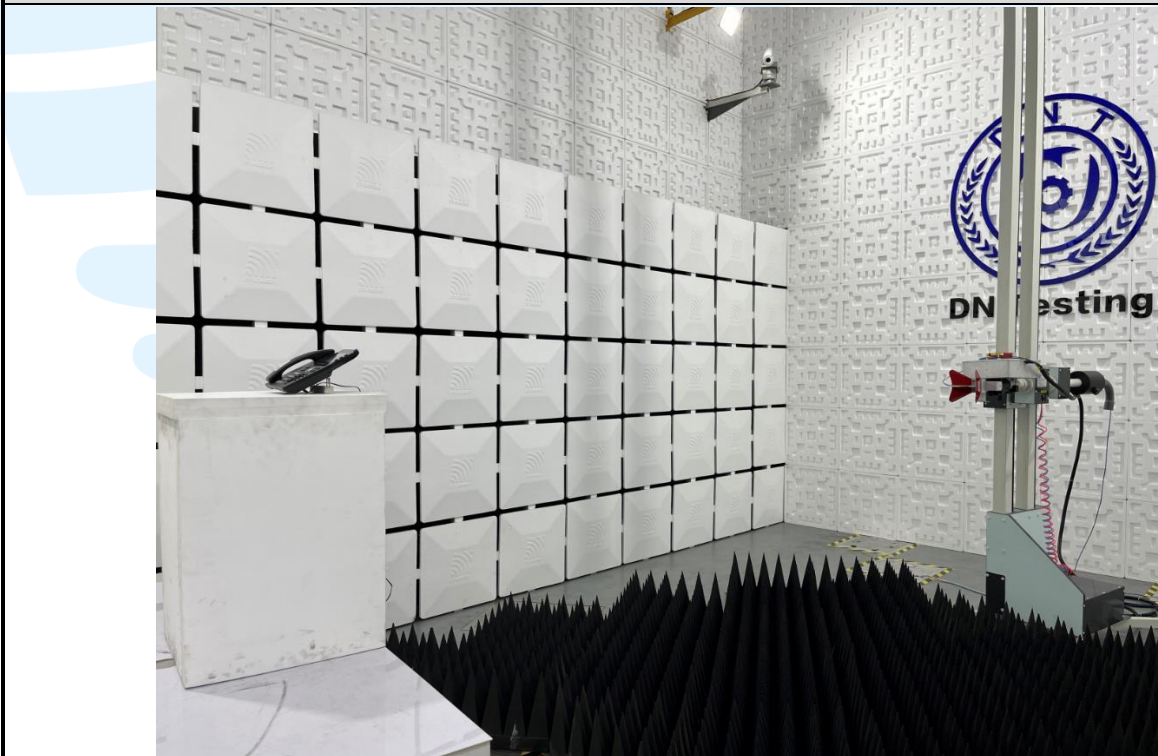
Radiated emission Test Setup (Above 1 GHz)
