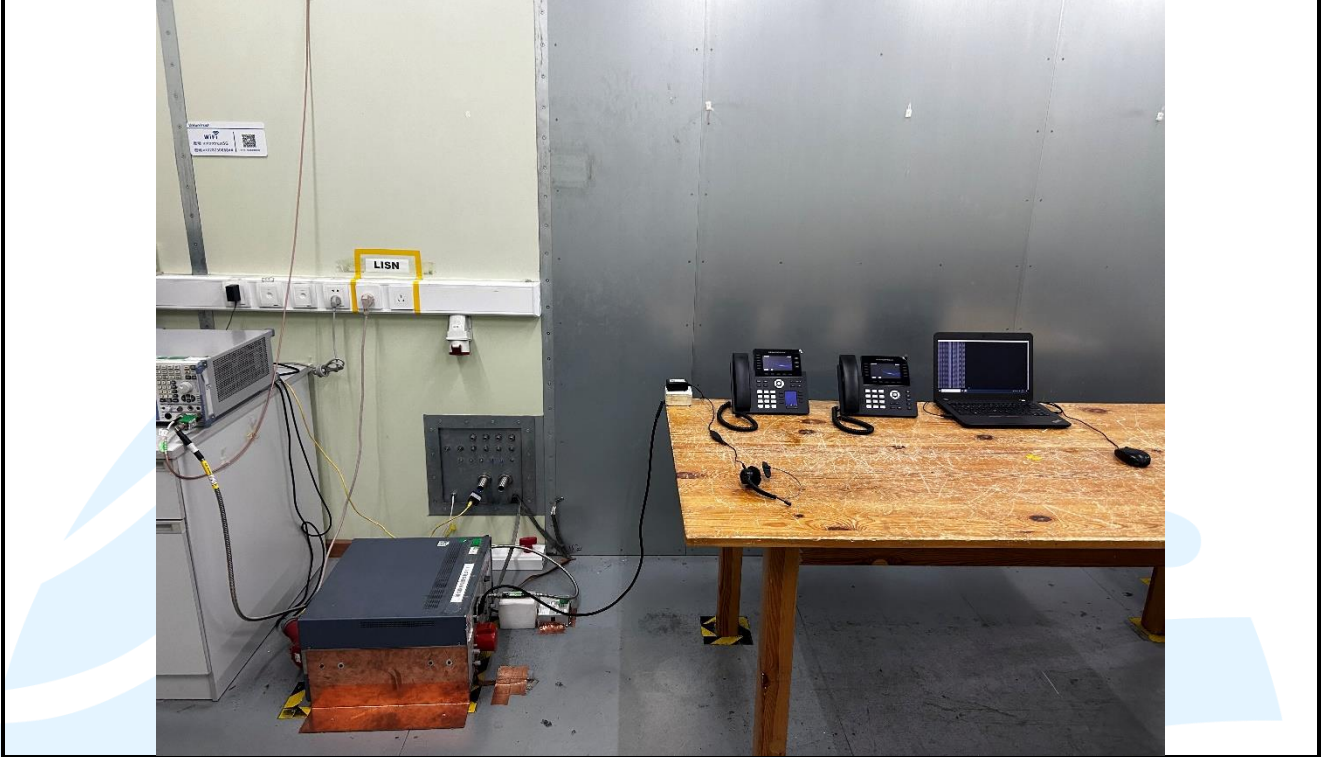
Conducted Emission Test Setup
