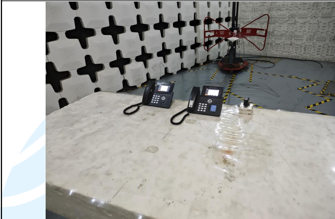
Radiated emission Test Setup-1 (30 MHz~1 GHz)
