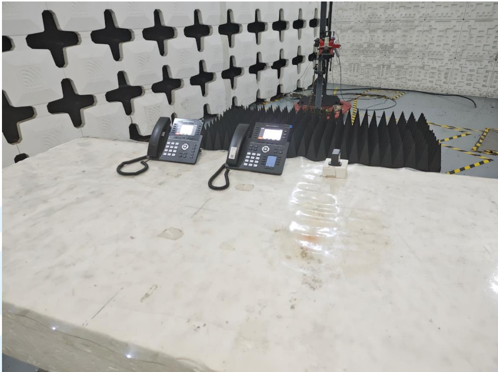
Radiated emission Test Setup-2 (Above 1 GHz)
