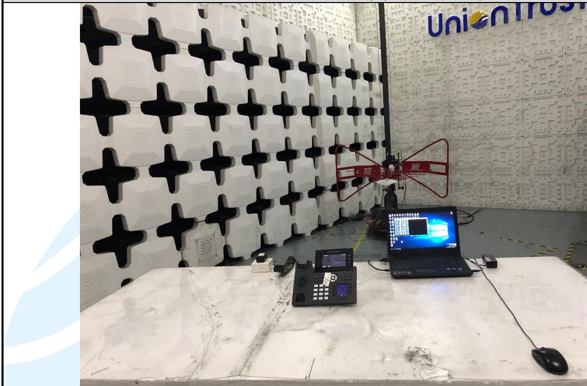
Radiated emission Test Setup (30 MHz~1 GHz)
