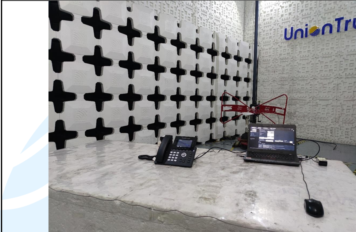
Radiated emission Test Setup (30 MHz~1 GHz)
