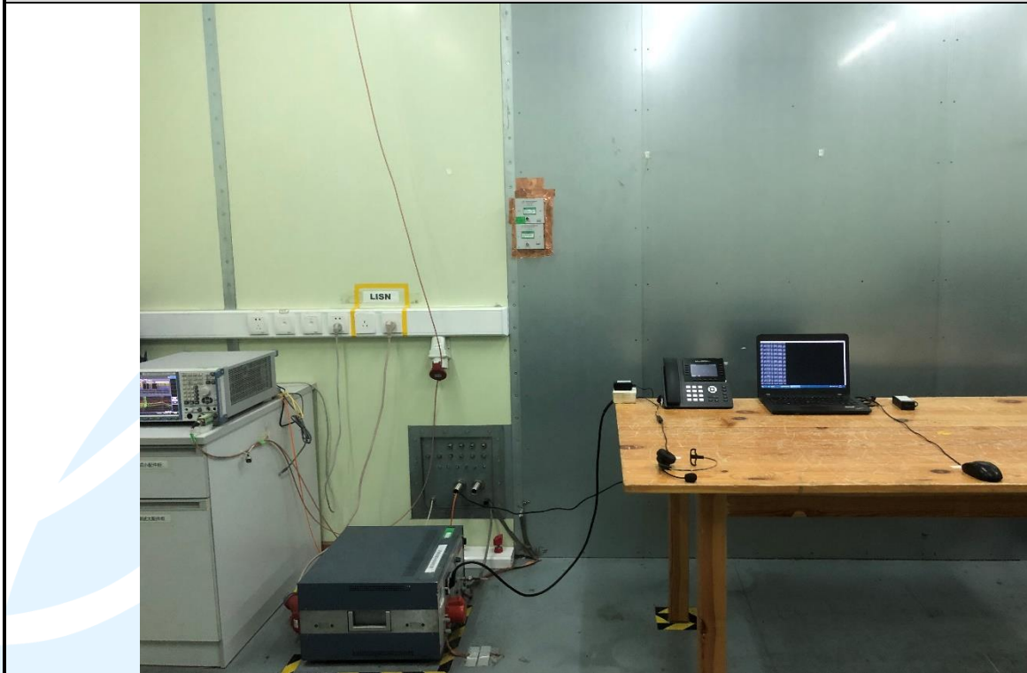
Conducted Emission Test Setup
