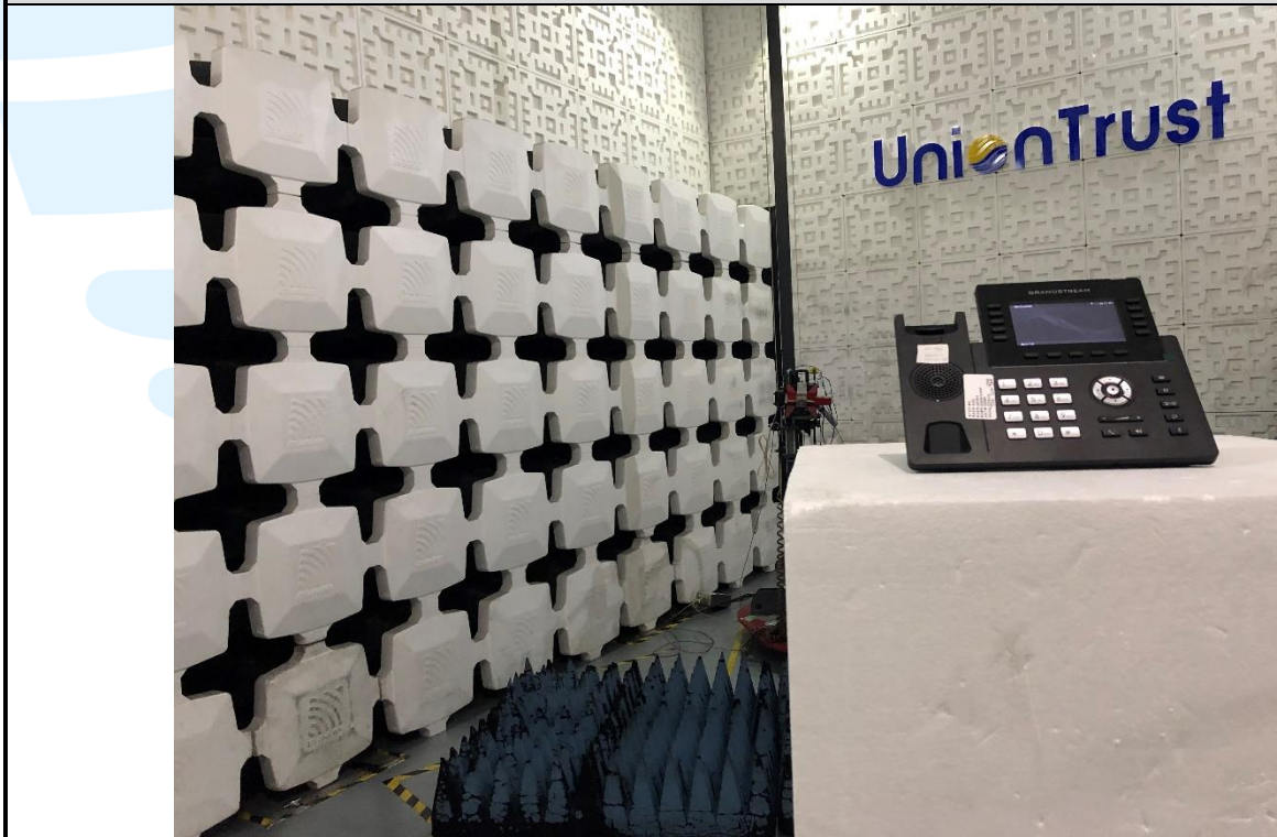
Radiated emission Test Setup (Above 1 GHz)
