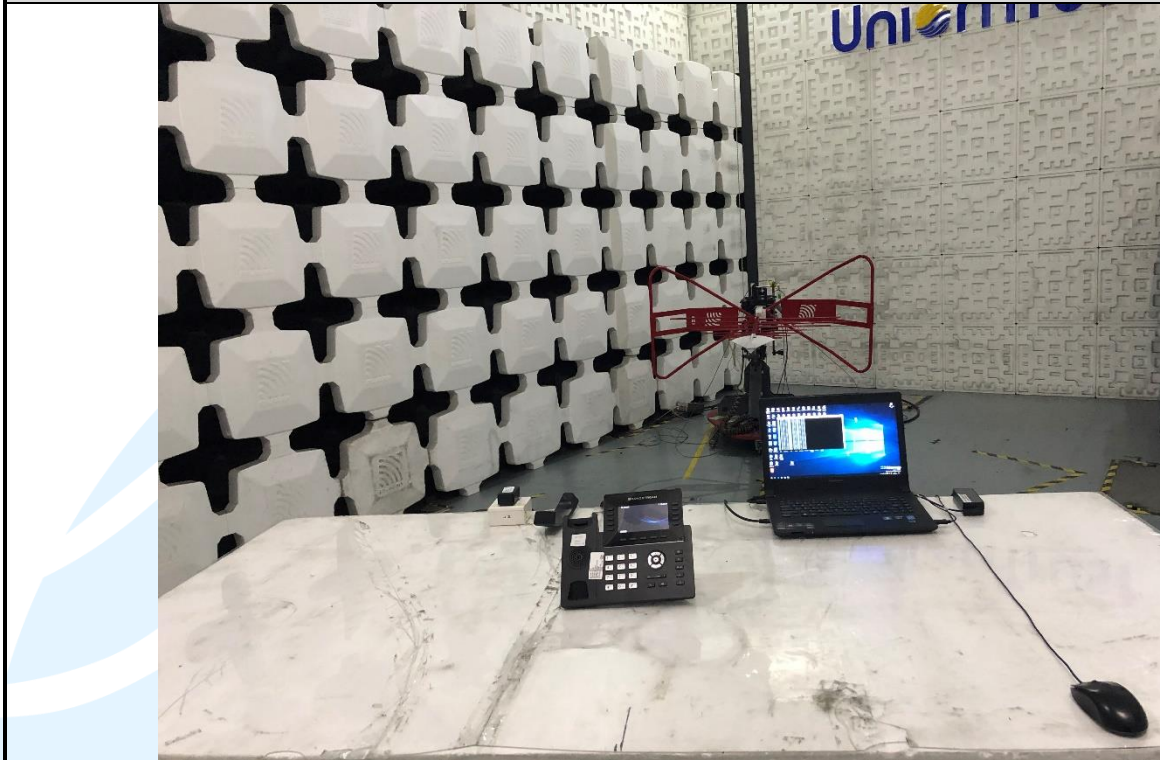
Radiated emission Test Setup (30 MHz~1 GHz)
