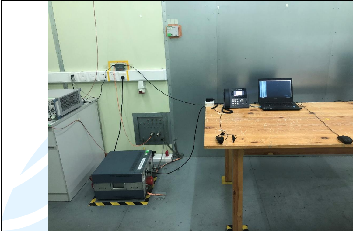
Conducted Emission Test Setup
