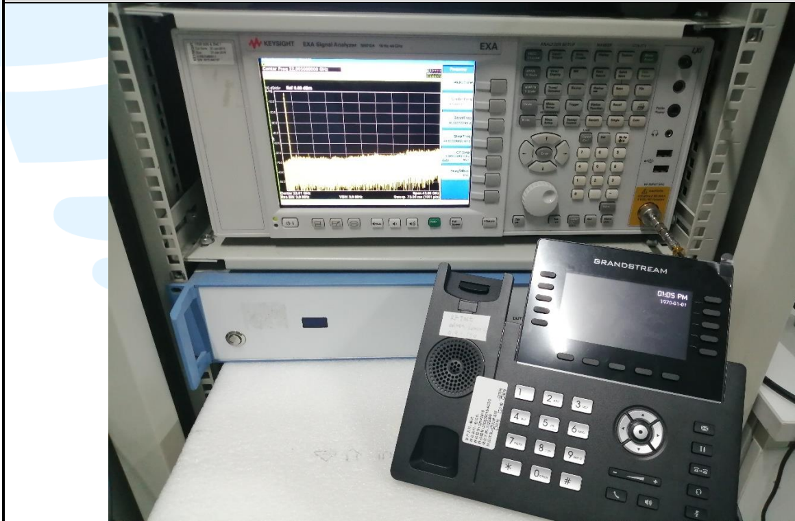
RF Conducted Test Setup
