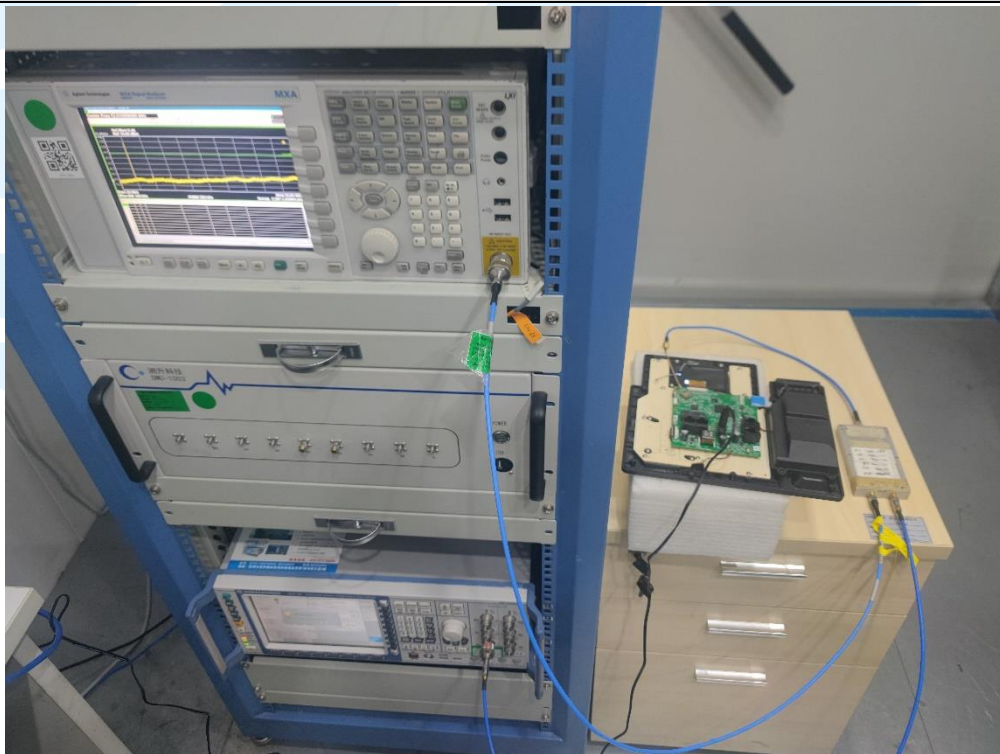
RF Conducted Test Setup
