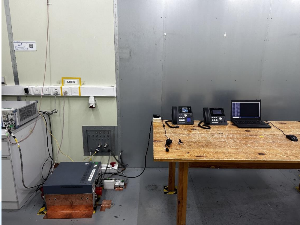
Conducted Emission Test Setup
