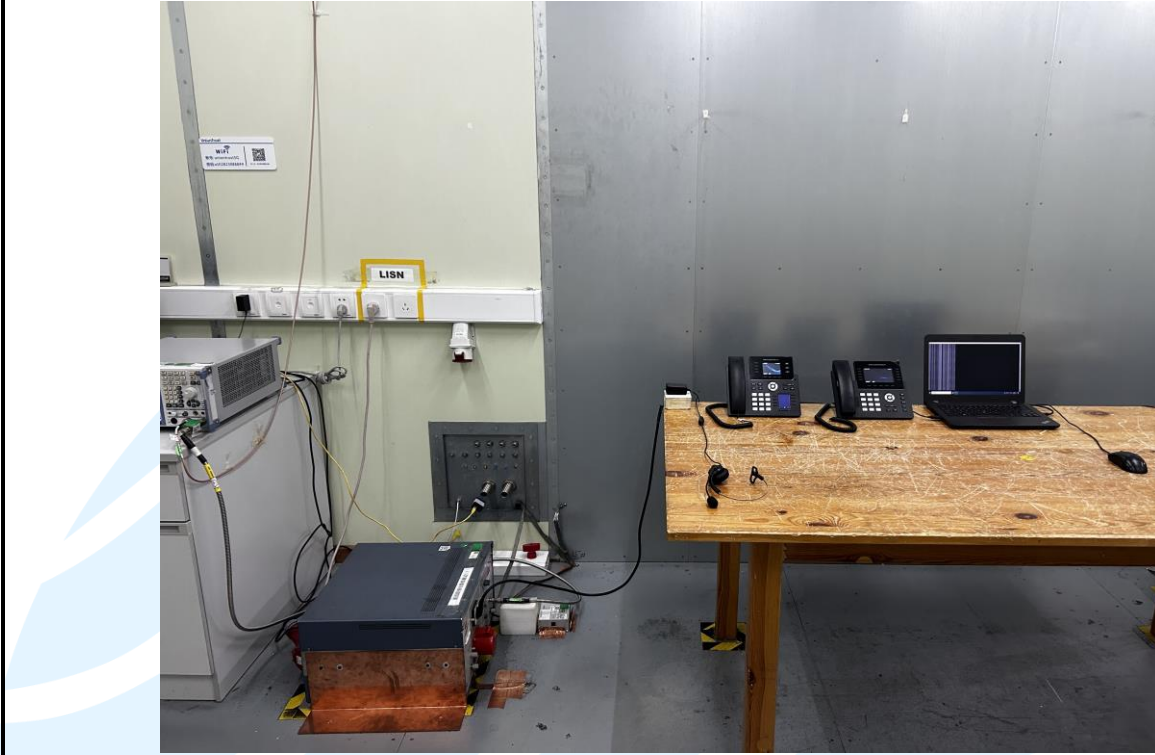
Conducted Emission Test Setup
