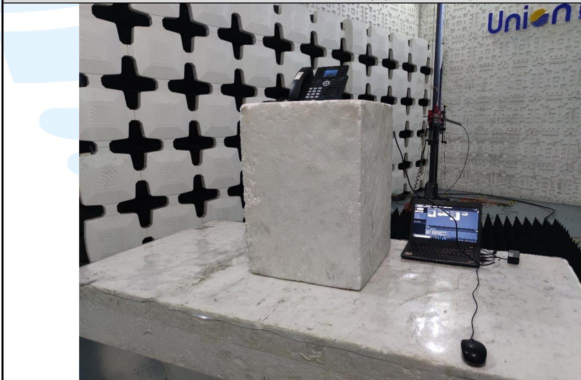
Radiated emission Test Setup (Above 1 GHz)
