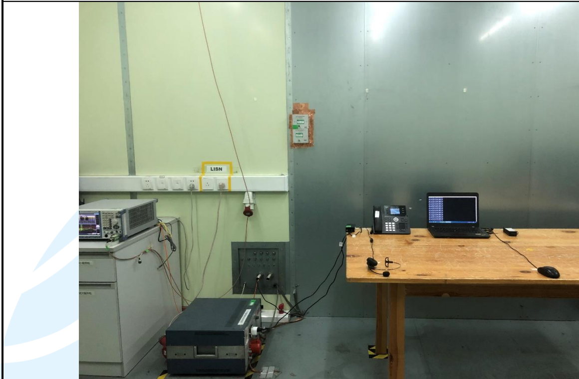
Conducted Emission Test Setup
