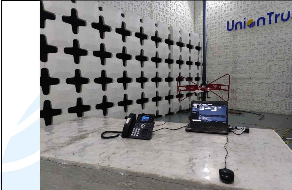
Radiated emission Test Setup (30 MHz~1 GHz)
