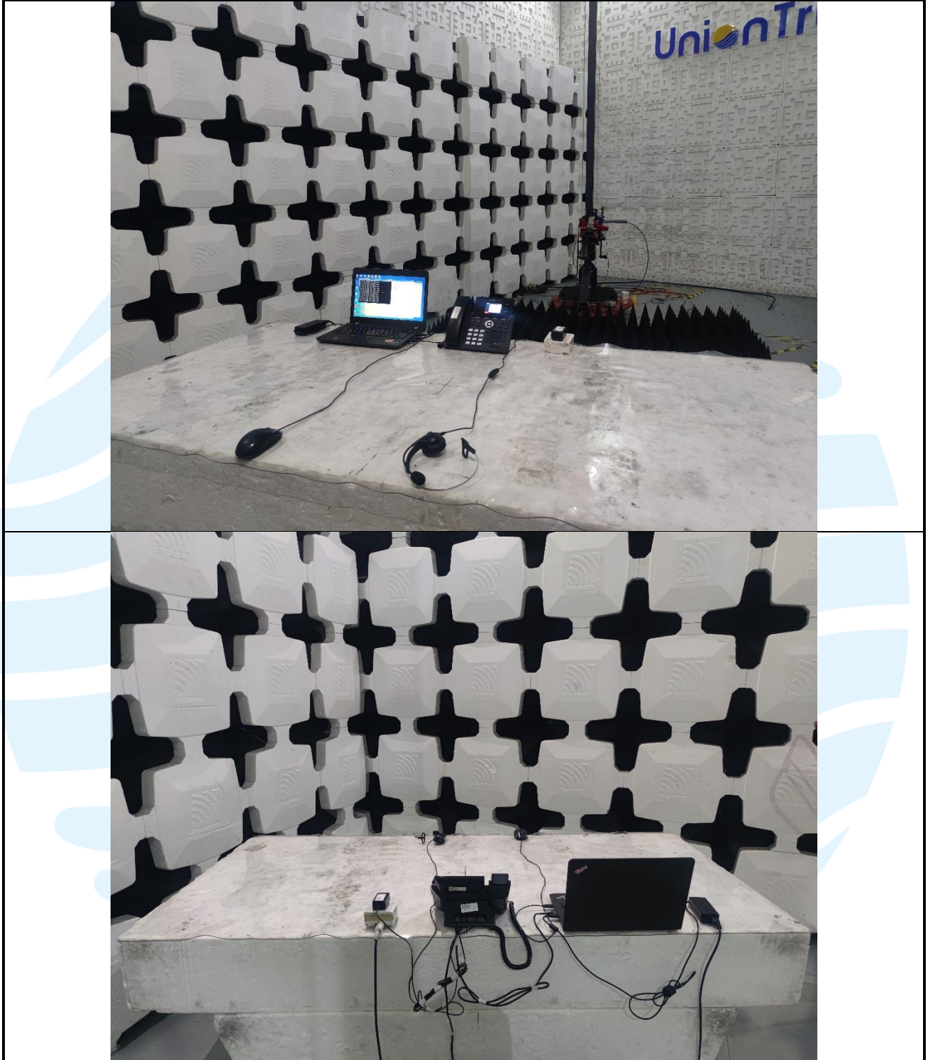
Radiated emission Test Setup-2 (Above 1 GHz)
