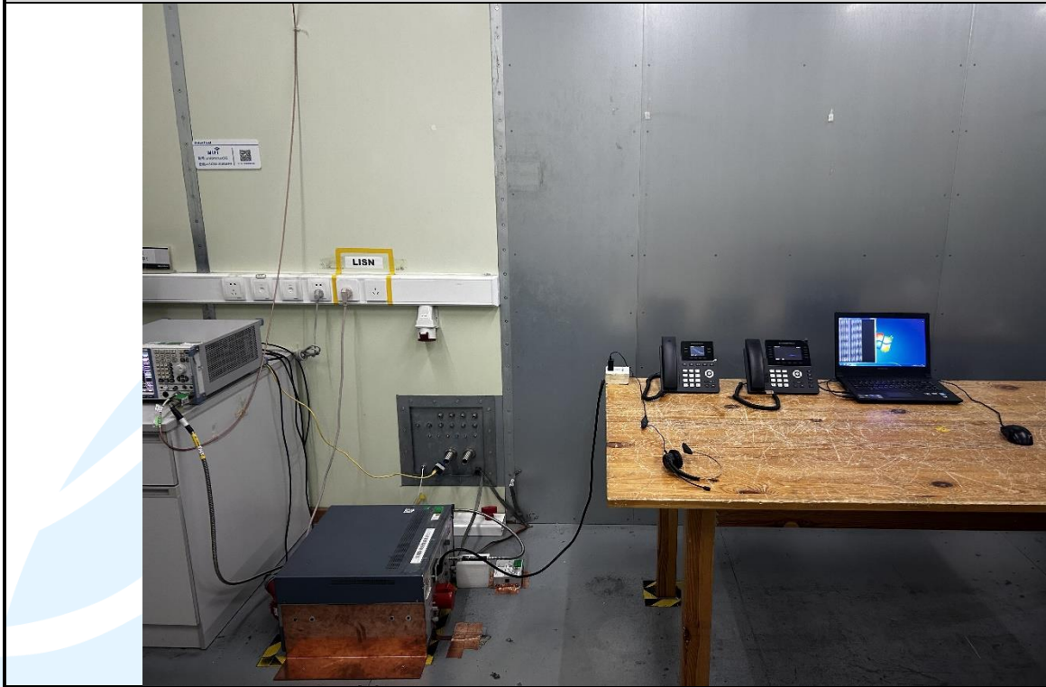
Conducted Emission Test Setup
