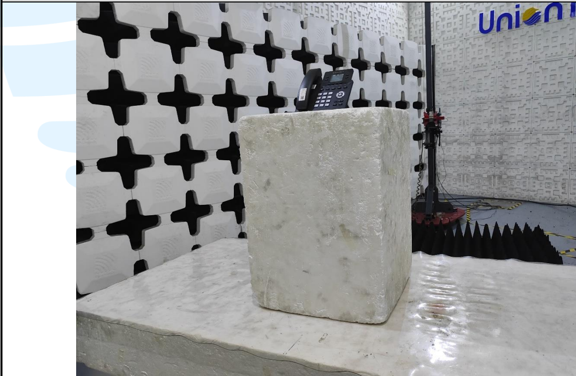
Radiated emission Test Setup (Above 1 GHz)
