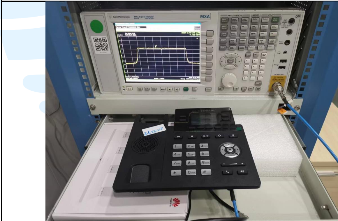
RF Conducted Test Setup
