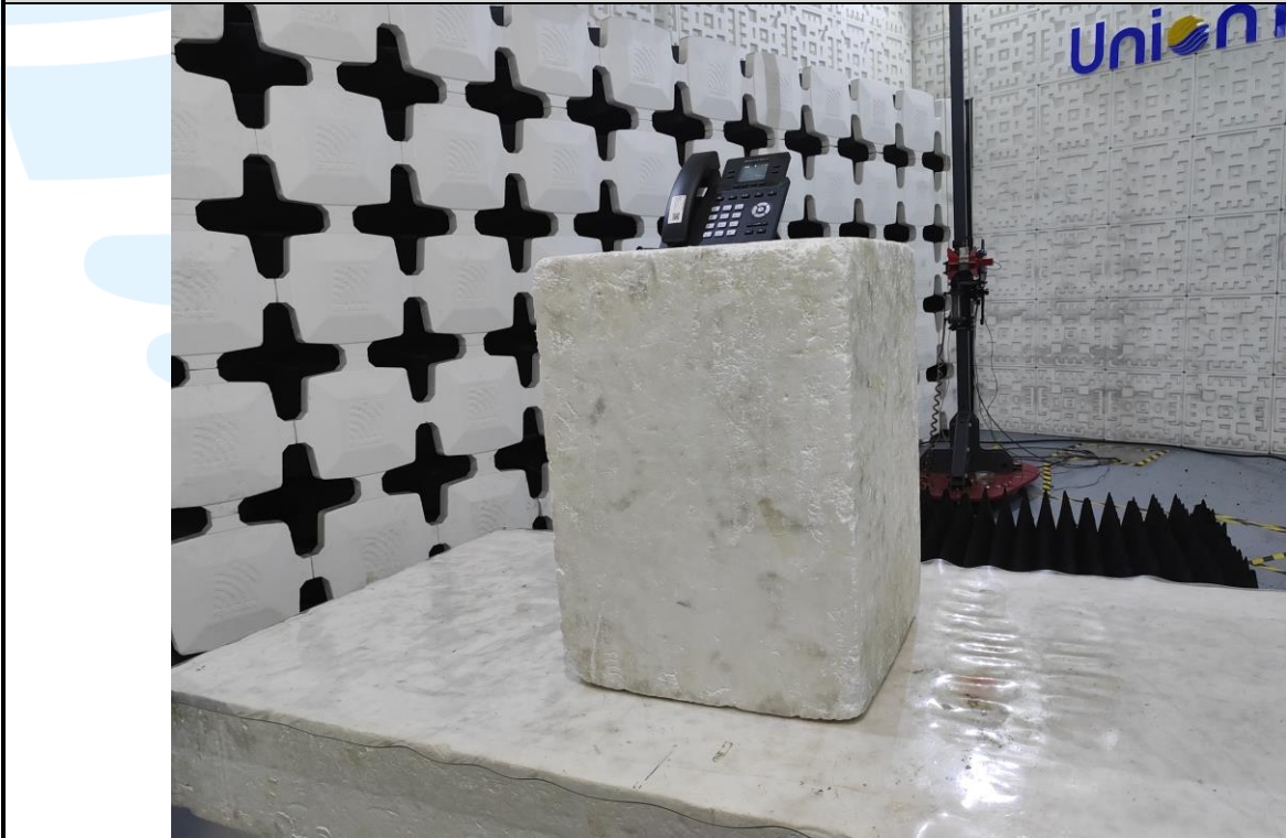
Radiated emission Test Setup (Above 1 GHz)
