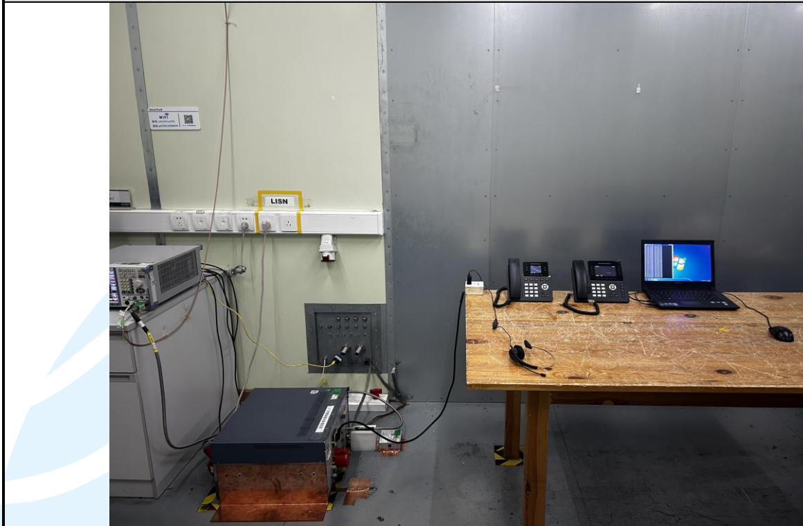
Conducted Emission Test Setup
