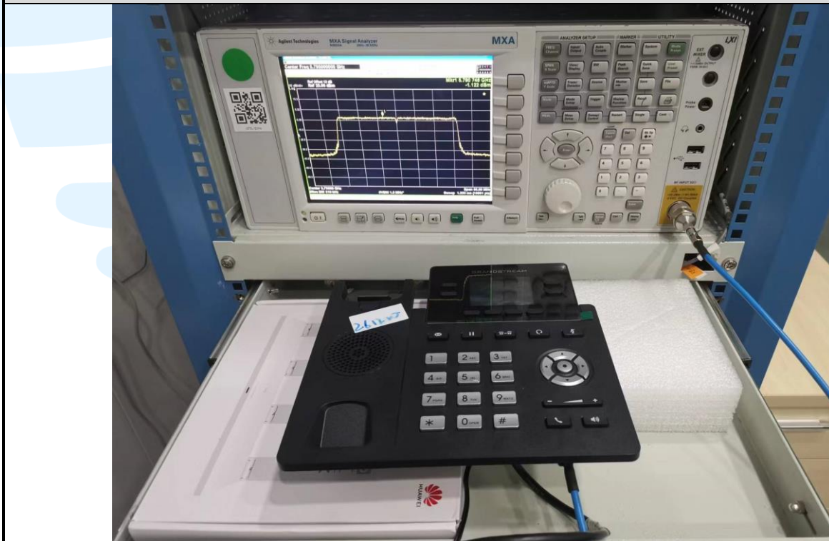
RF Conducted Test Setup
