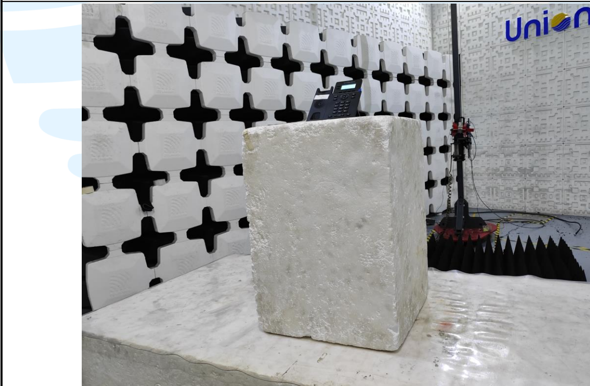
Radiated emission Test Setup (Above 1 GHz)
