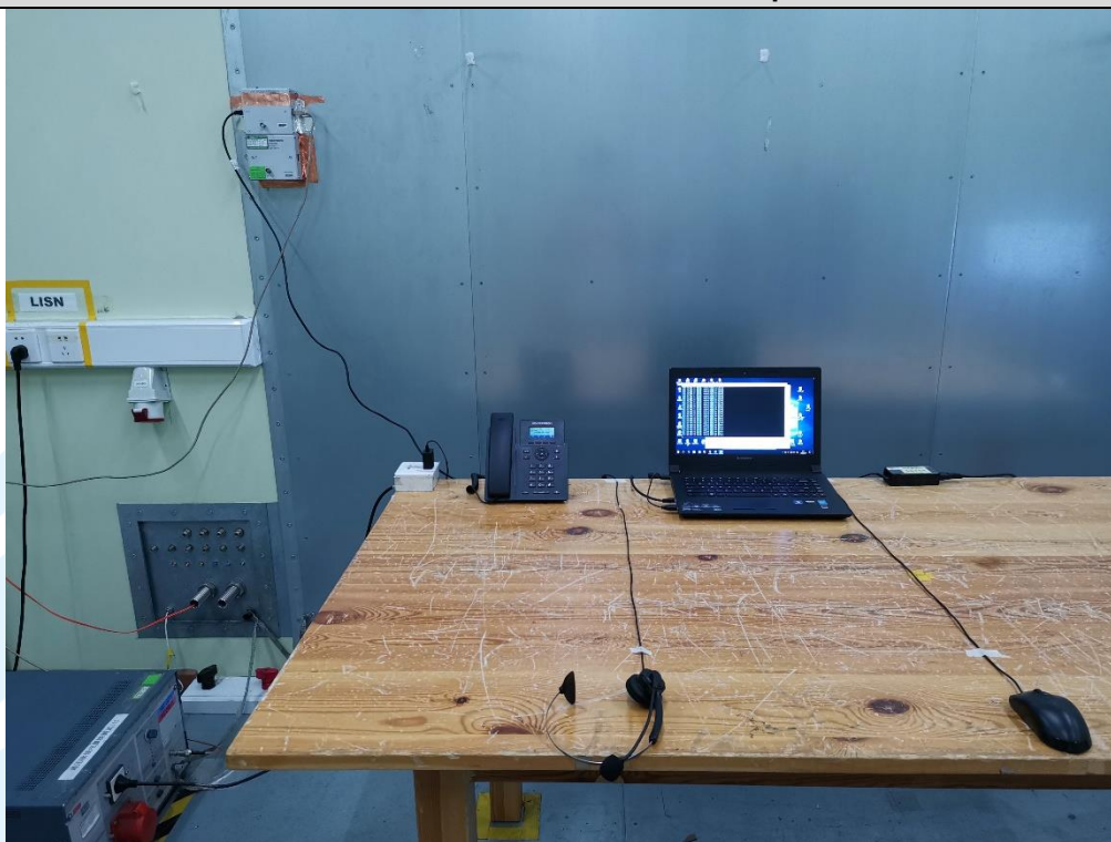
Conducted Emission Test Setup
