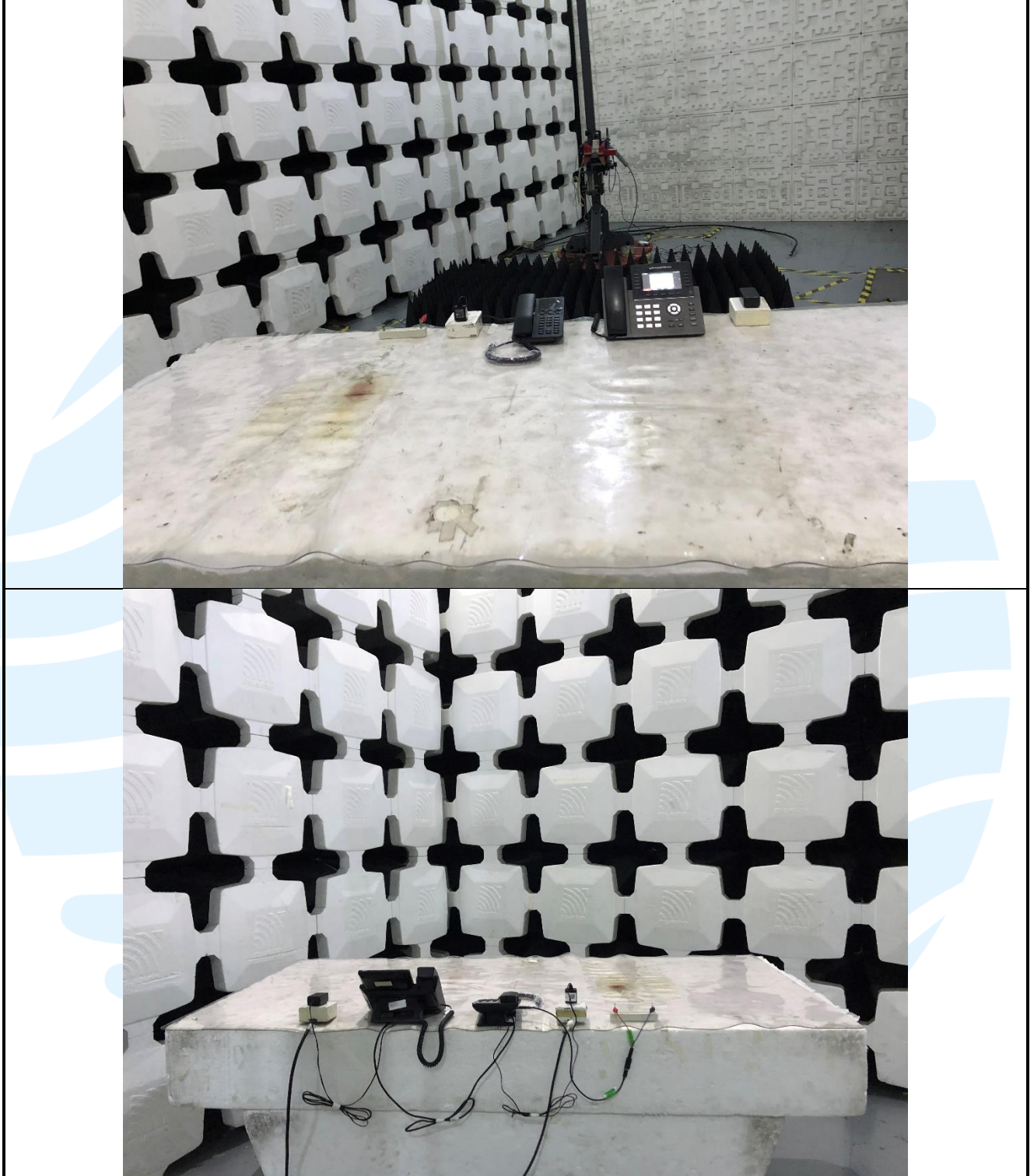
Radiated emission Test Setup-2 (Above 1 GHz)
