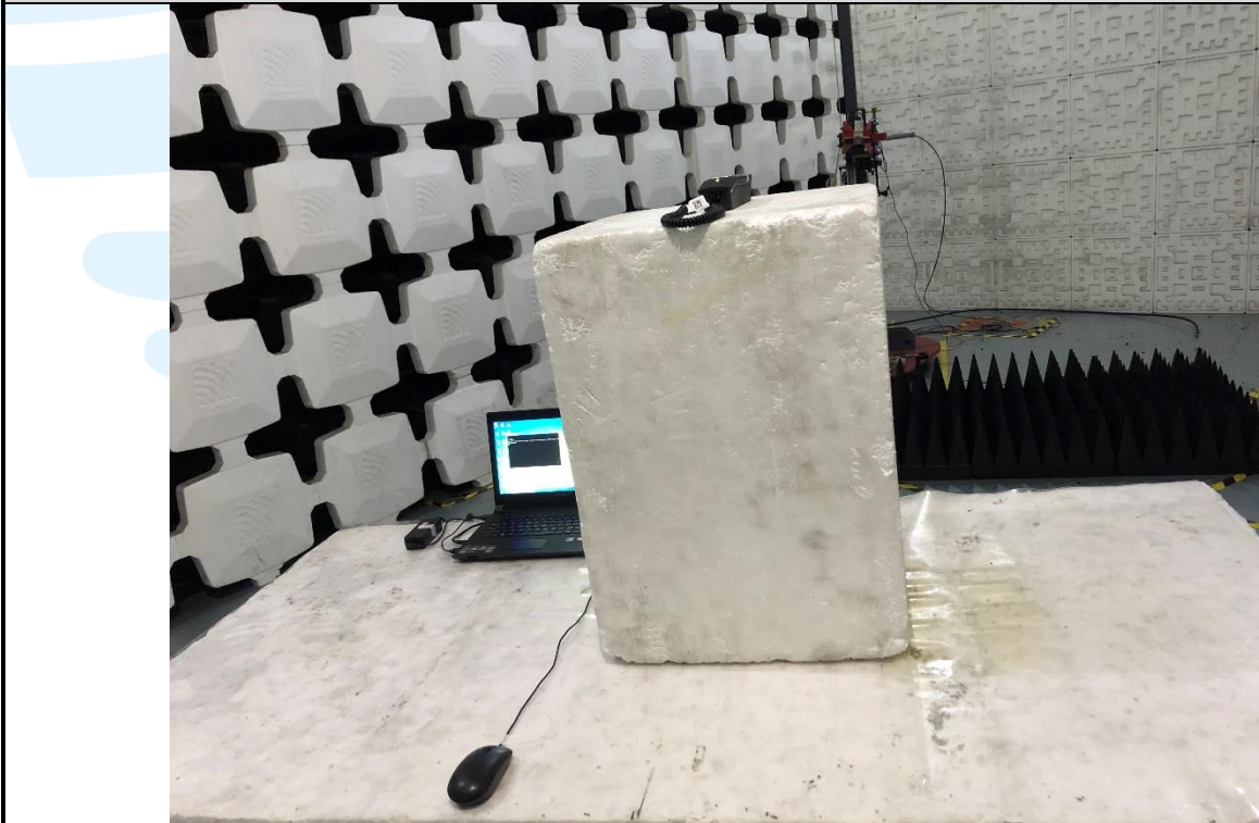
Radiated emission Test Setup (Above 1 GHz)
