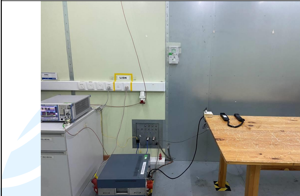
Conducted Emission Test Setup
