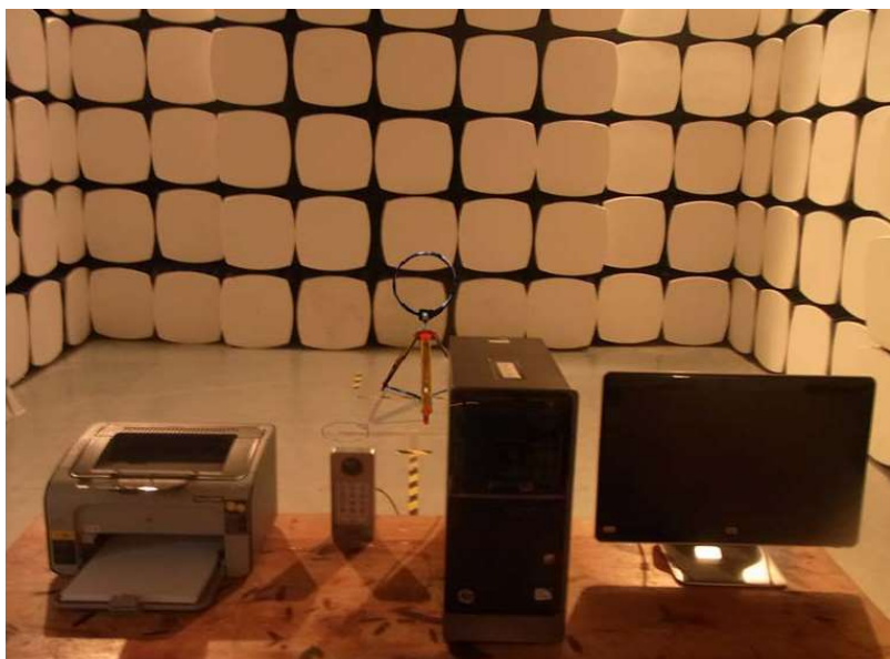
Radiated Emission Test Set-up :
