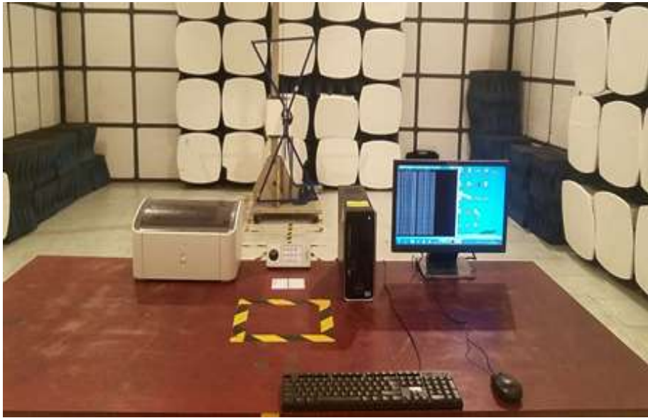
Radiated Emission Test Set-up(30-1000MHz)
