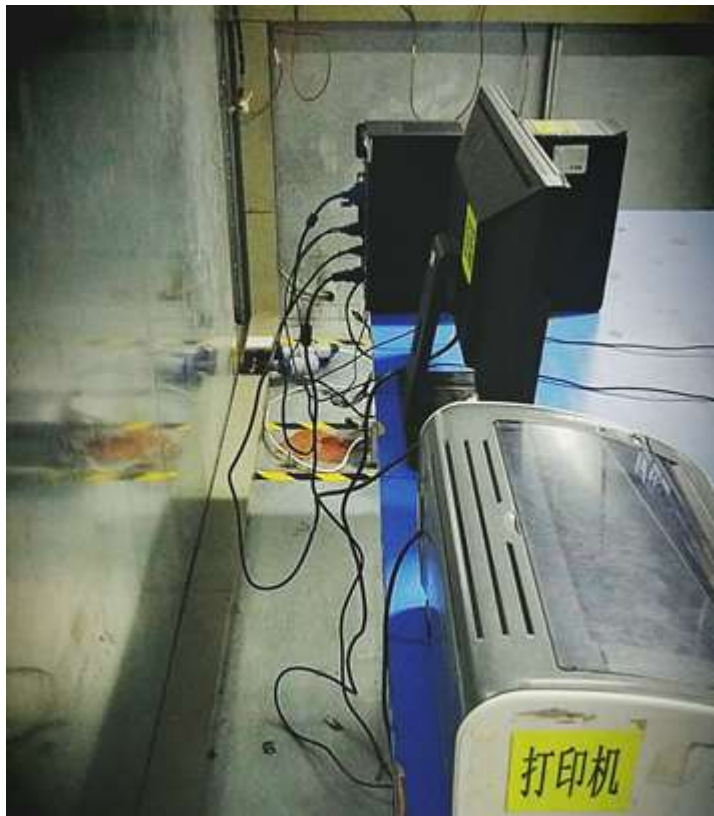
Conducted Emission Test Set-up –Back view
