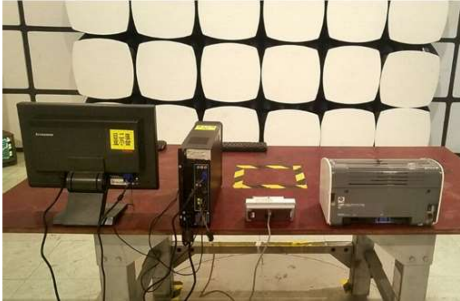
Radiated Emission Test Set-up-Rear View
