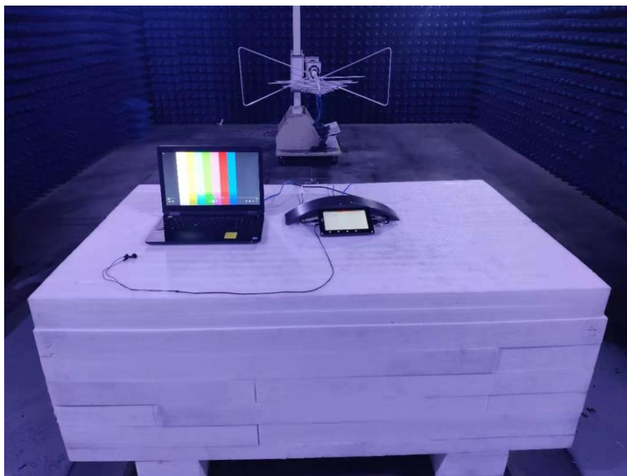
Photo of Radiated Emission Measurement (Below 1G)
